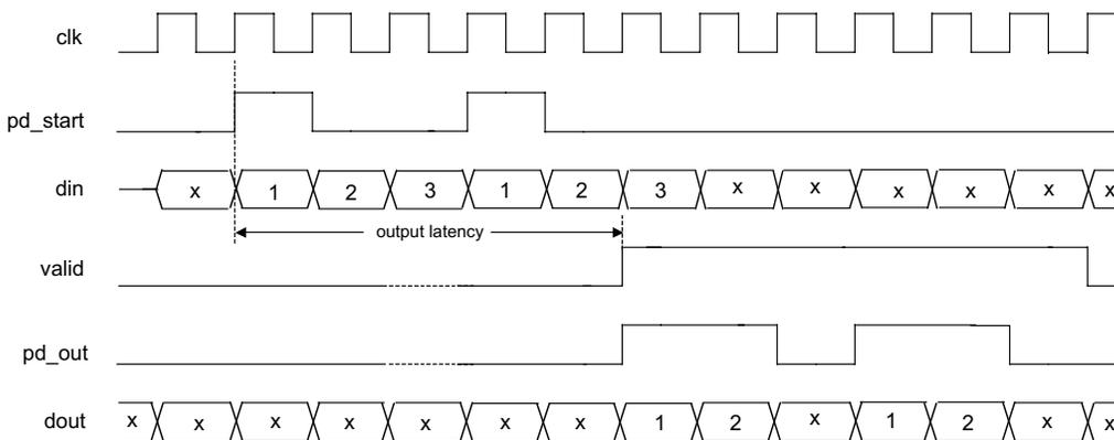
**Figure 9. Timing Diagram for a Hybrid (2 Cycles), Non-punctured Decoder**
