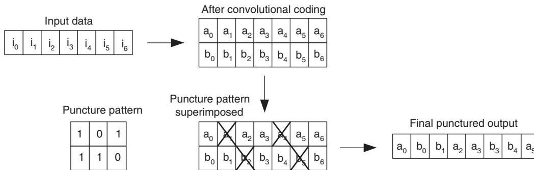
If puncturing is employed in the encoder, the decoder will have to “depuncture” the data before decoding. Depuncturing is done by inserting NULL symbols for the punctured symbols. NULL symbols are chosen to be equidistant from either '0' or '1'.
