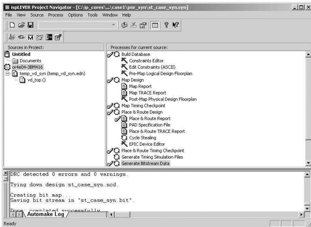
8. Double click on the **Constraint Editor**. You can enter the required preferences, including pin locking, using the constraint editor. You can also create an ASCII preference file using a text editor. For additional details on the ispLEVER preference language, refer to the ispLEVER online documentation.
