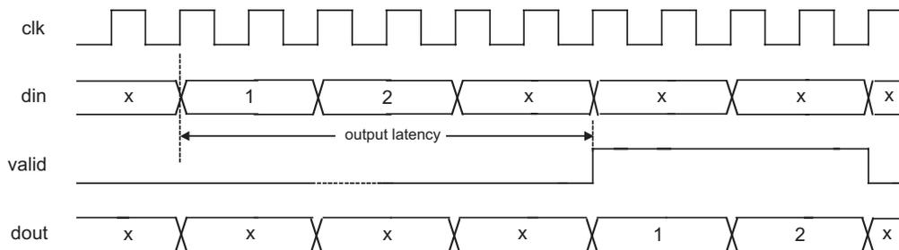
Figure 10. Timing Diagram for a Hybrid (2 Cycles), Punctured (Rate = 2/3) Decoder
