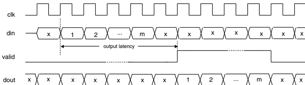
**Figure 8. Timing Diagram for a Parallel, Punctured (Rate = 2/3) Decoder**
