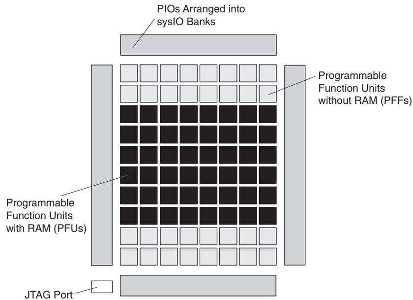
Figure 2-3. Top View of the LA-MachXO256 Device
