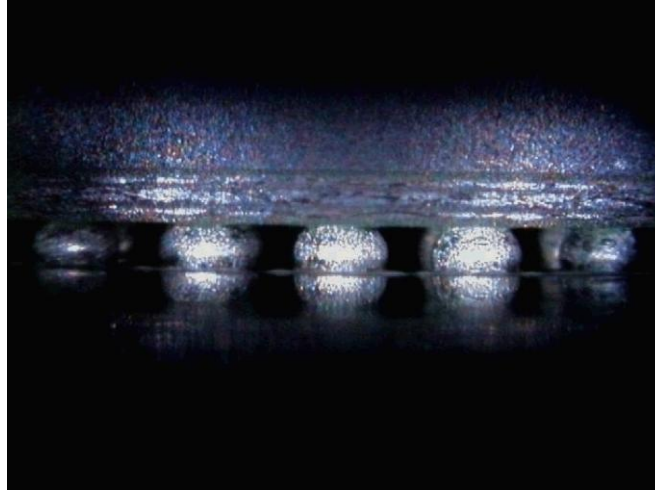
Figure 8.5. Edge View Camera Inspection
