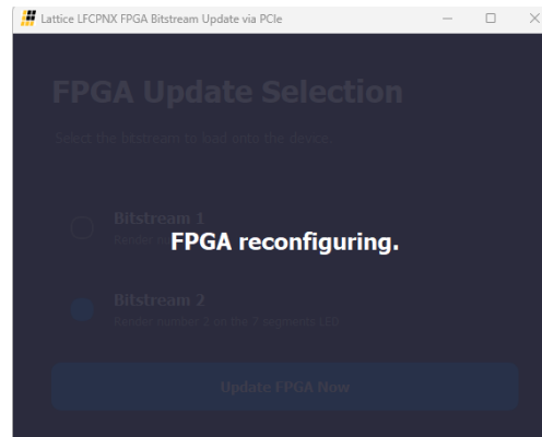
Figure 5.5. Automatic FPGA Reconfiguration Upon Successful Bitstream Update
