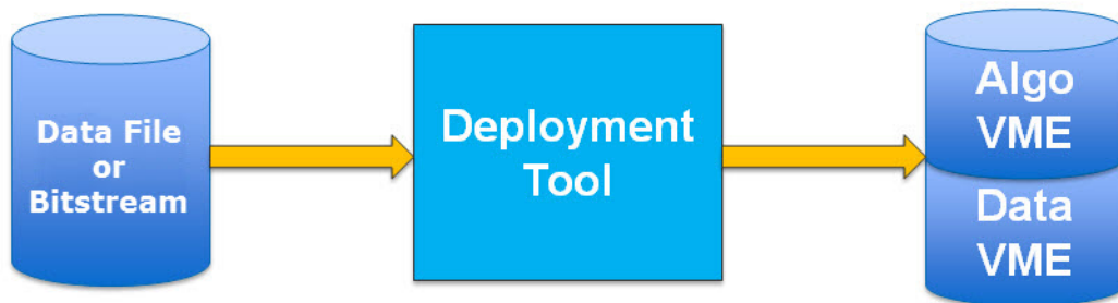
Figure 9: Full Embedded VME Flow
