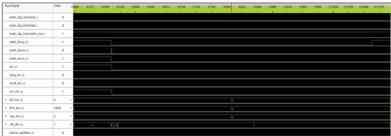
Figure 7.20. Reveal Analyzer Waveforms – End of First SEDC Scan with 2-bit Error Detection and Start of Next Scan
