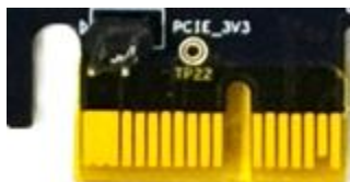
Figure 10.1. Top Side of PCIe Edge Connector
