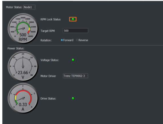
Figure 7.25. GUI Application Motor Status: RPM Lock Status When Target RPM is Achieved
