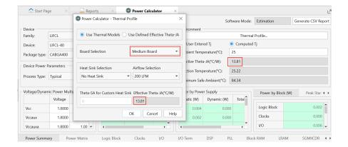
Change Board Selection to **Large Board** and the Effective Theta  $J_A$  value goes down from **13.81** to **11.92** The larger the board, the lower the Effective Theta  $J_A$  value. This is because you increased the area where the heat can spread out.
