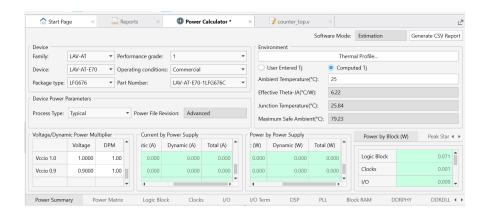
In the **Device** section, you can select the device, package, part name, performance grade, and operating conditions.
