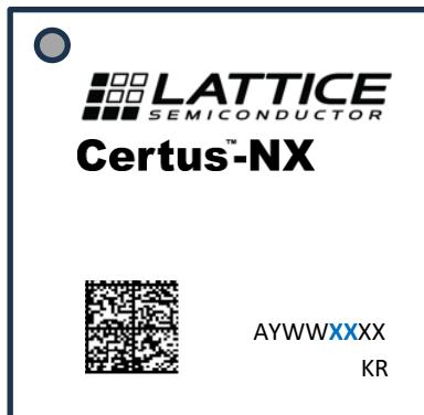
5<sup>th</sup> character in the Datecode will be “7” (for wirebond) or “P” (for WLCSP) and 6<sup>th</sup> character will be “P” indicates devices built and tested at SFA Semicon Ltd. Korea.
