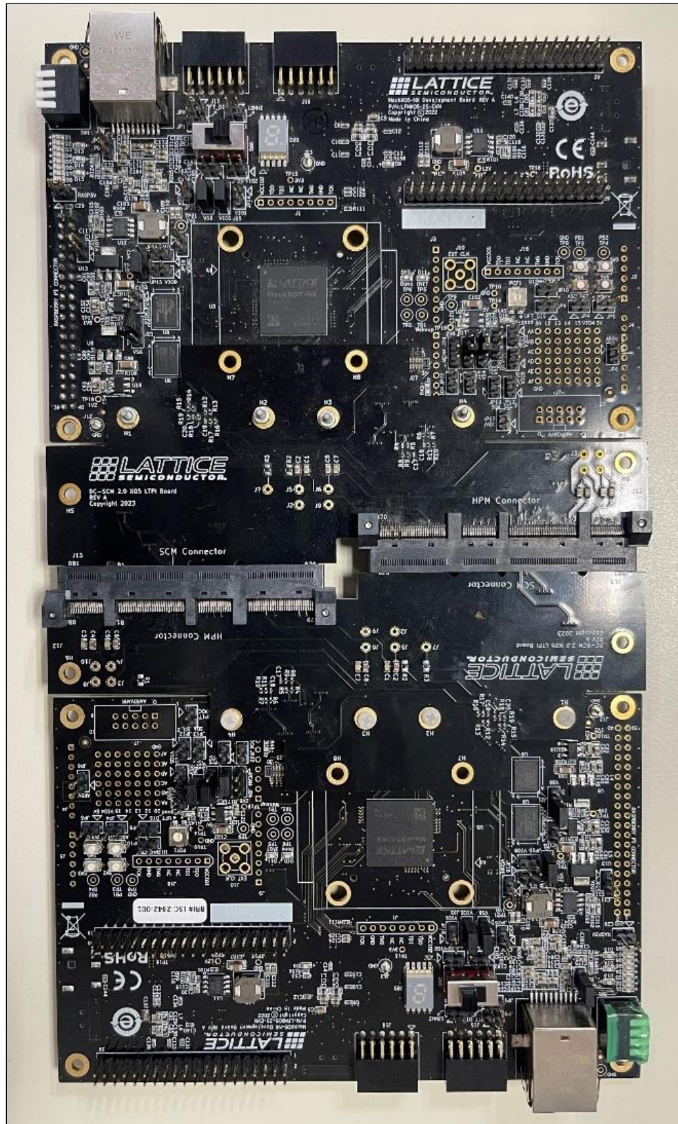
Figure 5.3. MachXO5-NX LTPi Adaptor Board with MachXO5-NX Development Board
