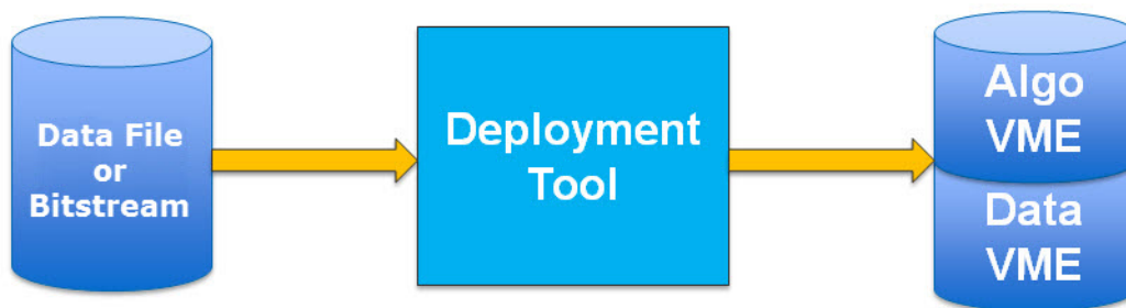
Figure 9: Full Embedded VME Flow
