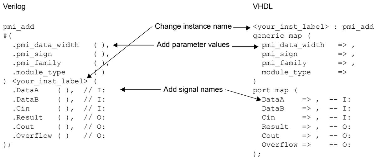
5. If using stand-alone synthesis and simulation tools, add the PMI soft IP from the `<install_path>/ip/pmi/` directory.
