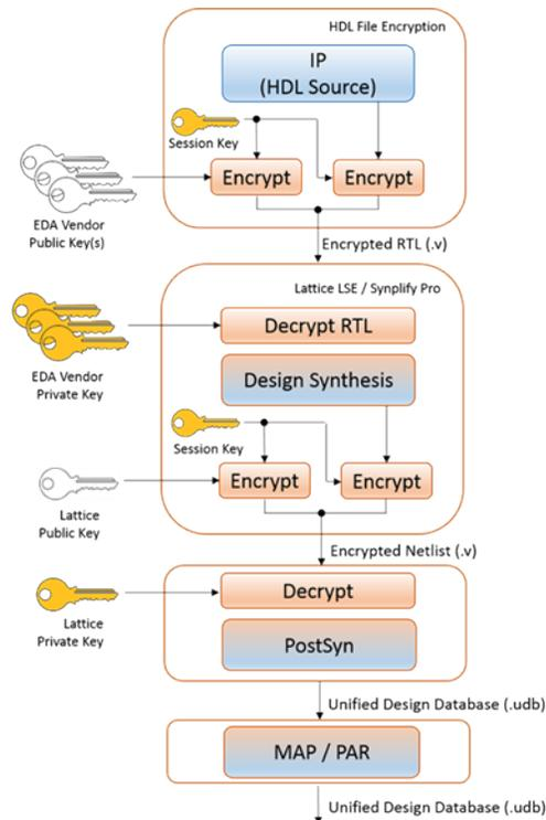
The encryption flow uses symmetric and asymmetric encryption methods to maximize the design security. The symmetric method only involves a single symmetric key for both, encryption and decryption. The asymmetric method involves the public-private key pair. The public key is published by a vendor and is used by the Radiant software. The private key is never revealed to the public.
