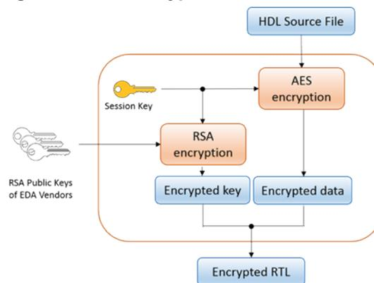
By separating the encryption of data and key, you can use public keys from different vendors to encrypt the same HDL file.
