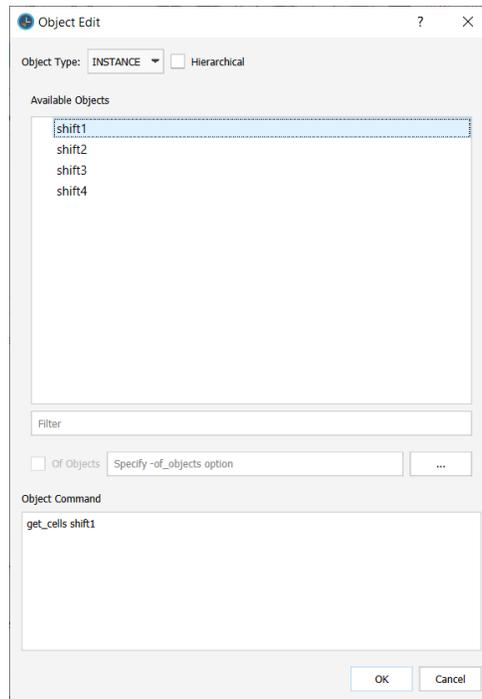
In the example above, **shift1**, **shift2**, **shift3**, and **shift4** are **Instance Names**. The command is **get\_cells** as shown in the **Object Command** pane.
