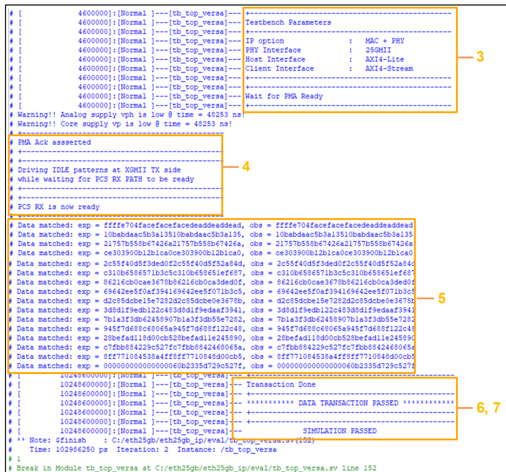
Figure 6.32. Example Design Simulation Output for Non-Continuous Mode
