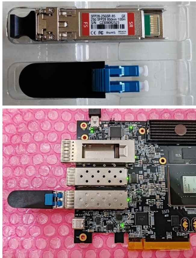
Figure 6.35. Loopback Module Setup
