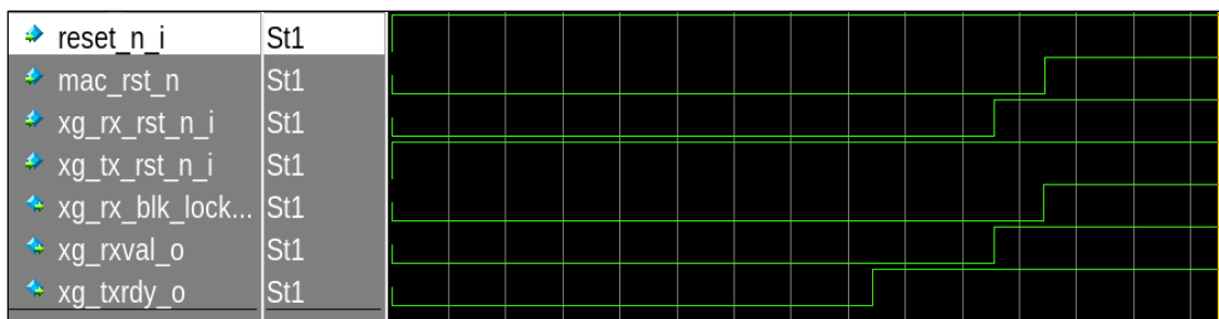
Figure 2.42. Example Testbench Reset Waveform
