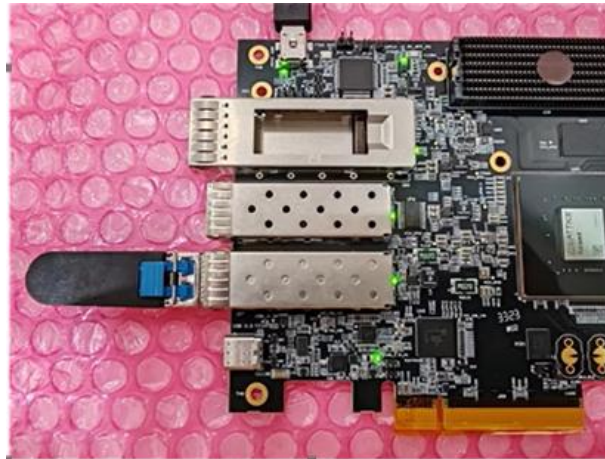
Figure 6.38. Loopback Module Setup
