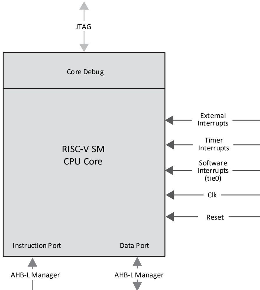
Figure 2.2. RISC-V SM CPU Core Block Diagram
