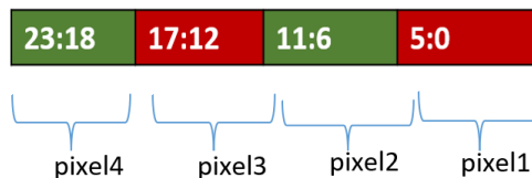
Figure 2.7. Bit Allocation for BPP=6 and PPC=4 for Bayer RGGB input
