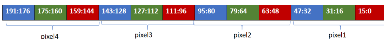
Figure 2.10. Bit Allocation for BPP=16 and PPC=4 for RGB input
