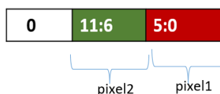
Figure 2.6. Bit Allocation for BPP=6 and PPC=2 for Bayer RGB input
