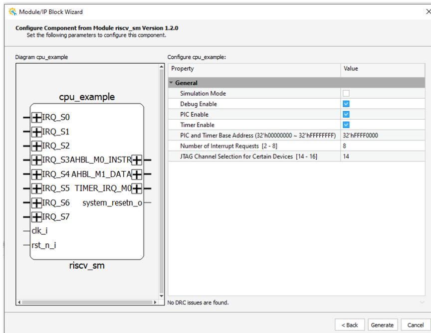
Figure 3.2. Configuring Parameters
