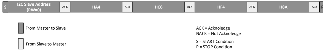
Figure 6.12. Slave I 2 C Configuration Activation Flow
