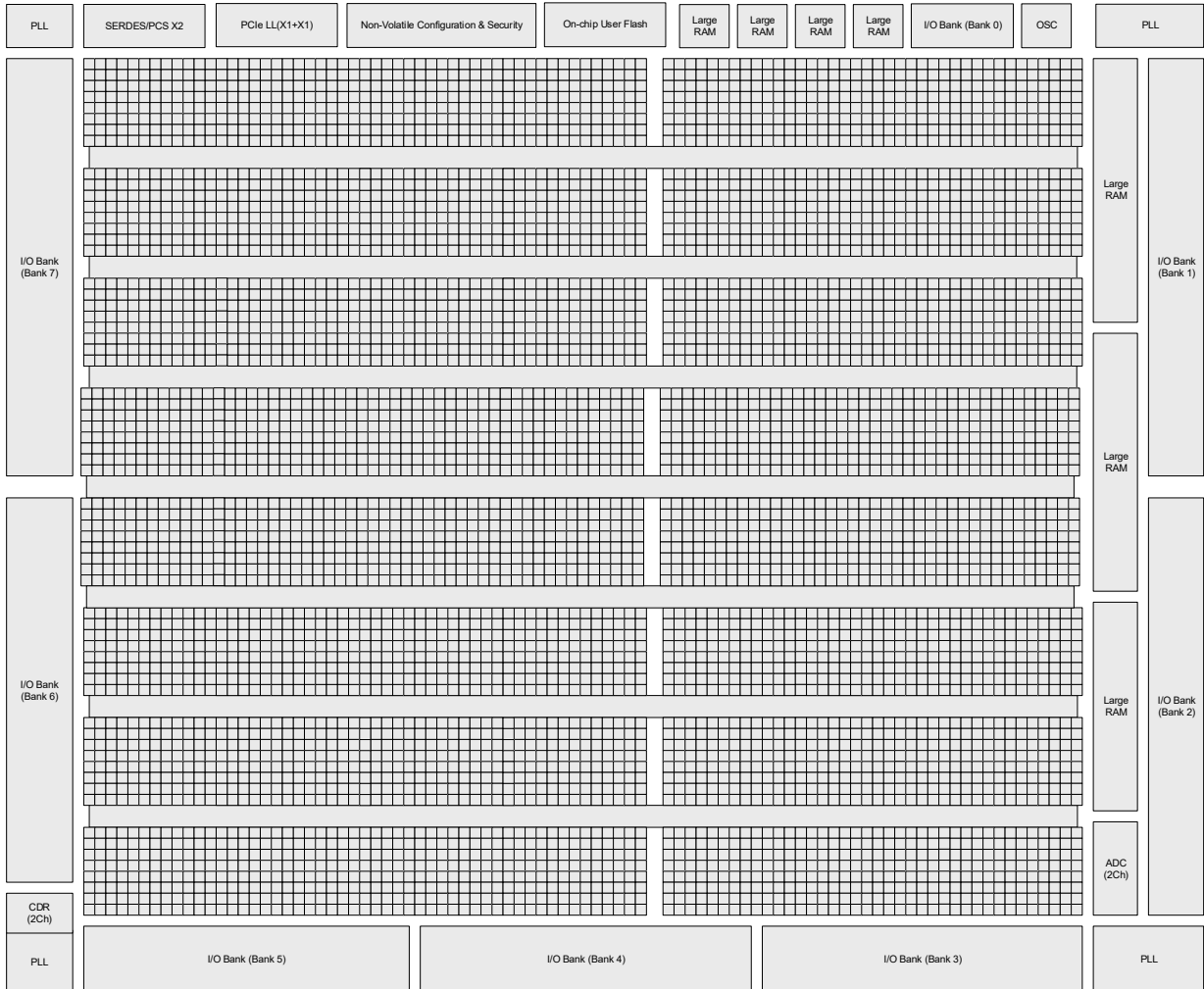
Figure 2.3. Simplified Block Diagram, MachXO5-NX-100T Device (Top Level)
