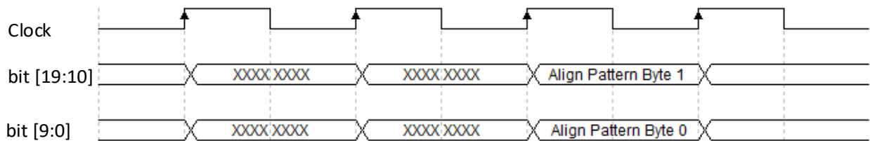
Figure 6.13. After 2-byte Boundary Alignment
