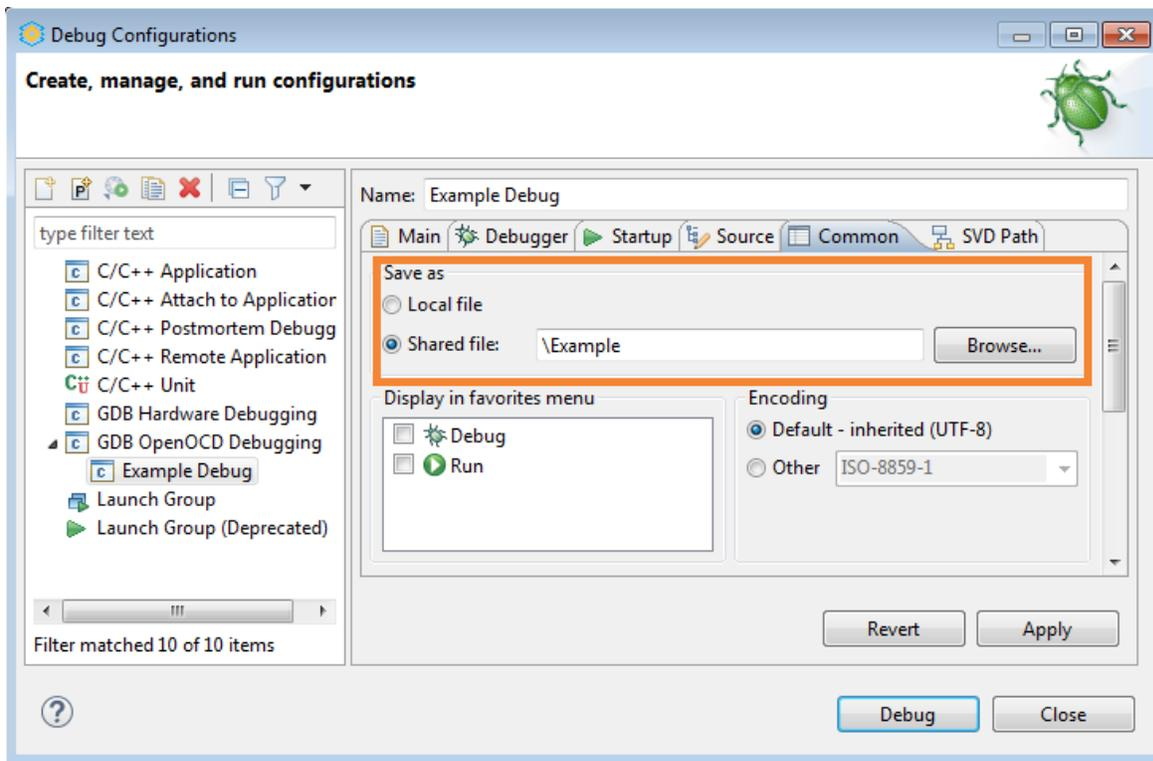
Figure 3.35 Common Tab of Debug Configurations
