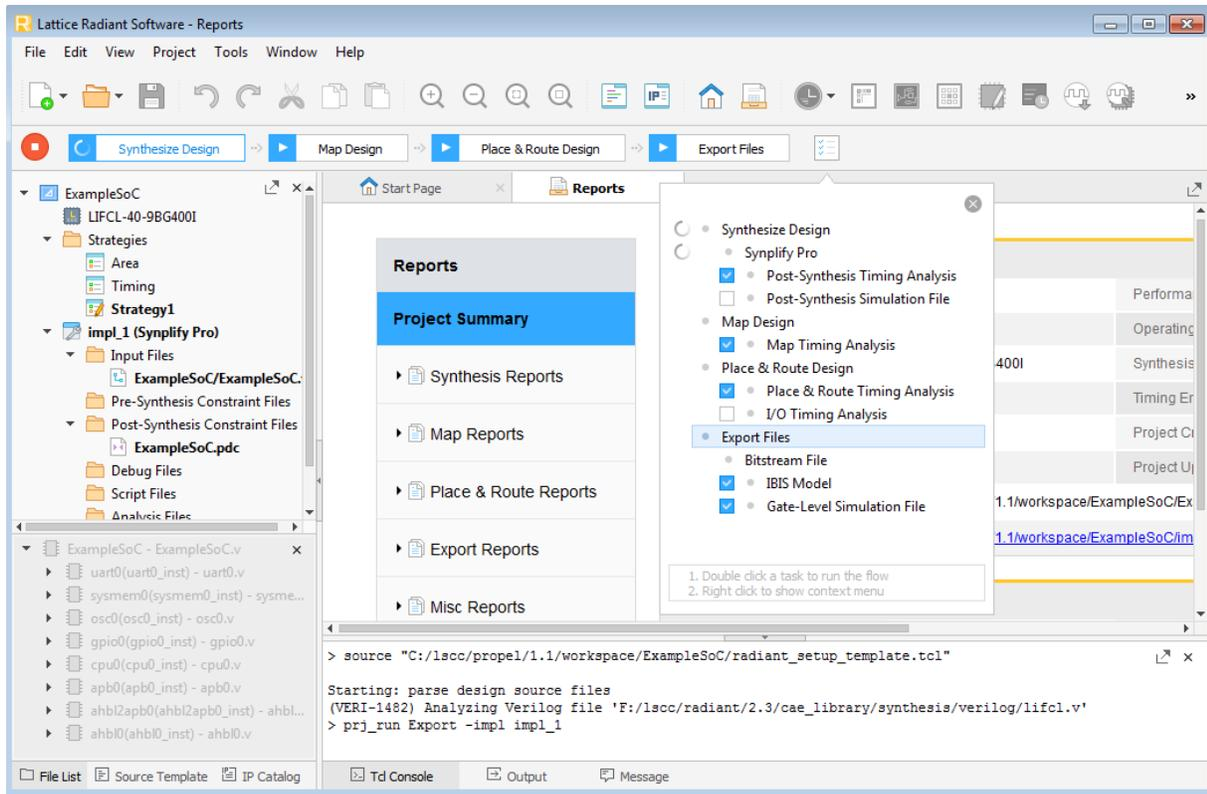
Figure 3.15. Generate Programming File in Lattice Radiant
