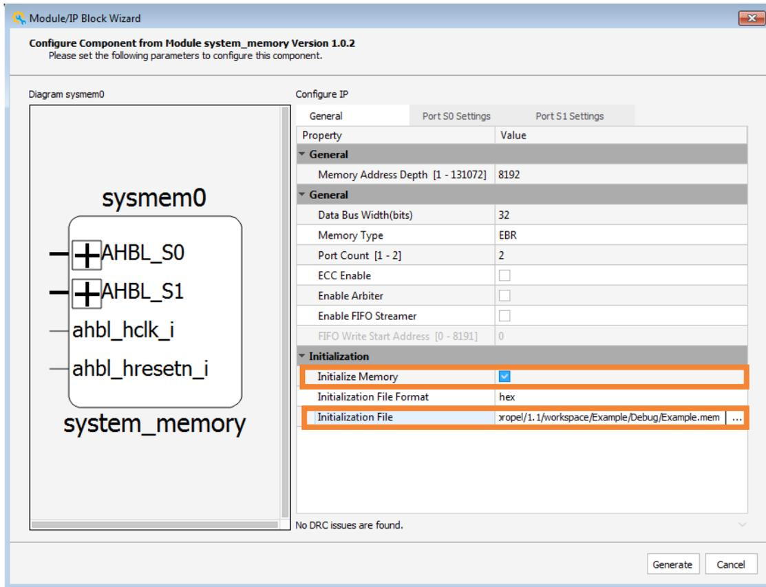
Figure 3.29. Configure Module System Memory
