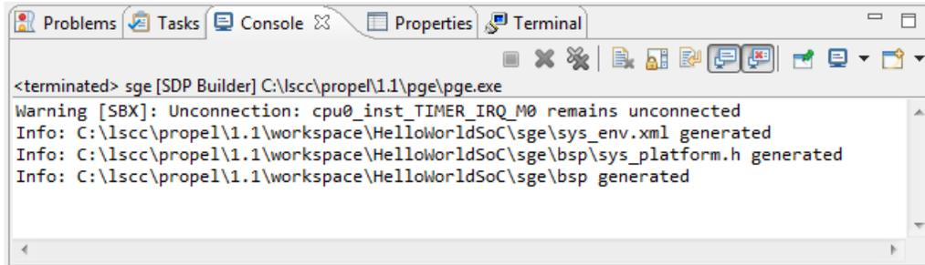
Figure 4.7 Build Result of HelloWorld SoC Project
