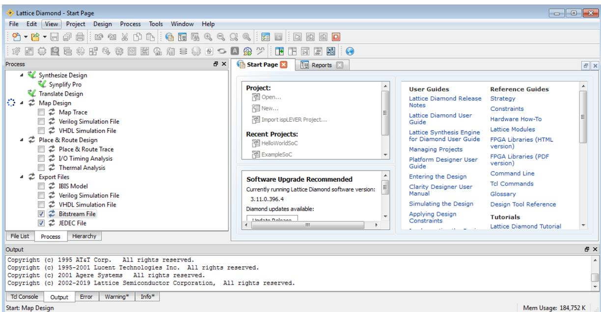
**Figure 3.14. Generate Programming File in Lattice Diamond**
