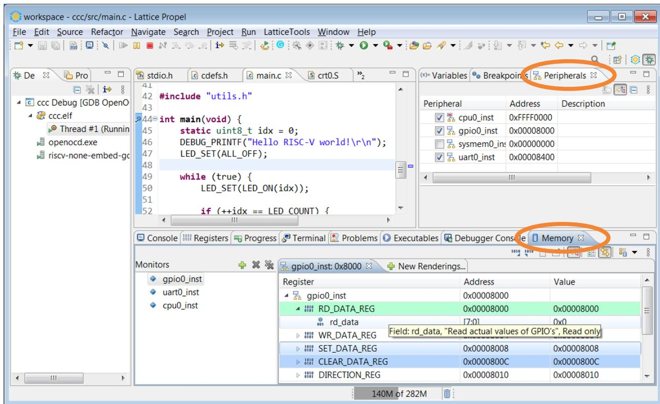
Figure 3.38 Peripherals View in Debug Perspective
