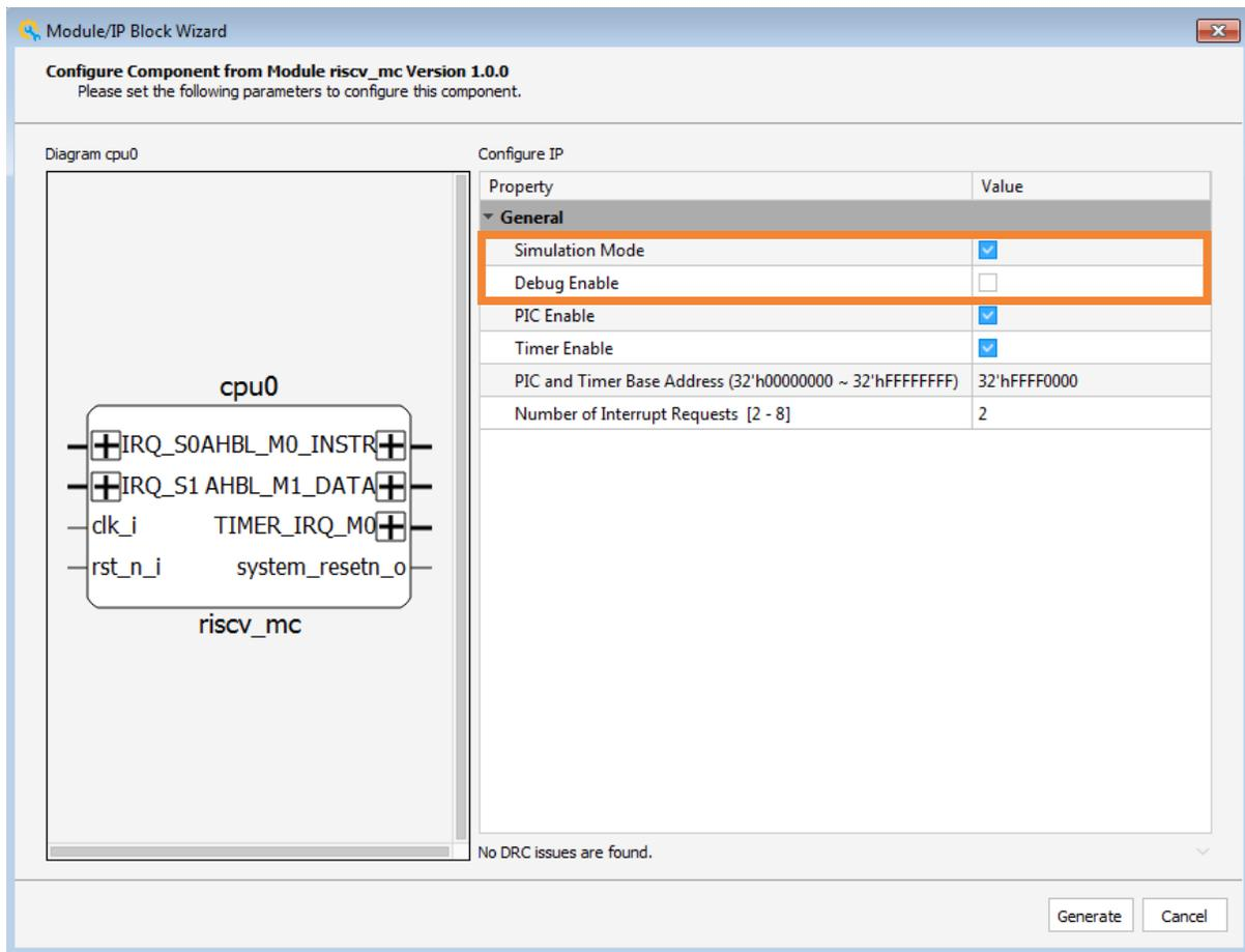
Figure 3.28. Configure Module RISC-V MC
