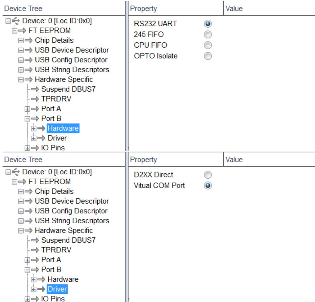
**Figure 4.2 Configure the FTDI Device**
