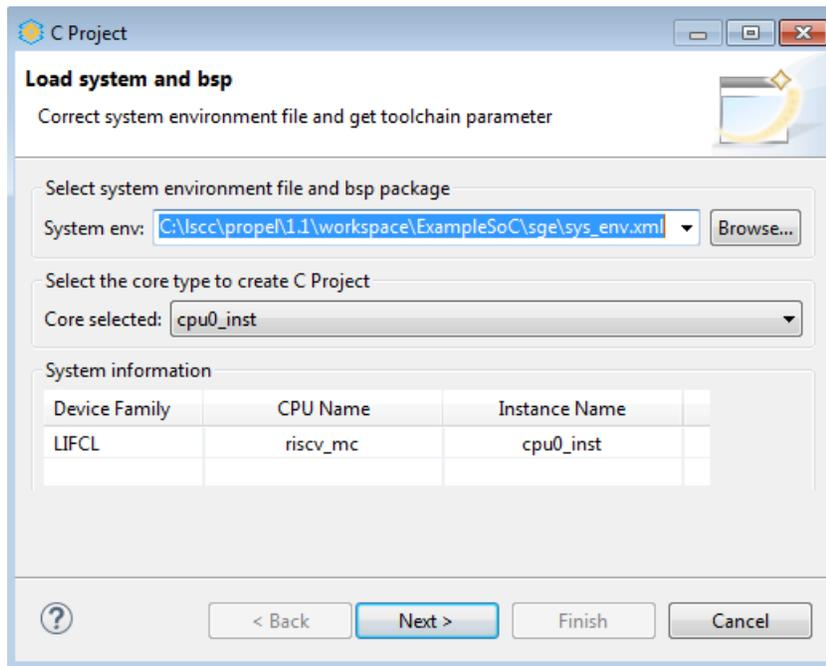
Figure 3.18. Load System and BSP Dialog
