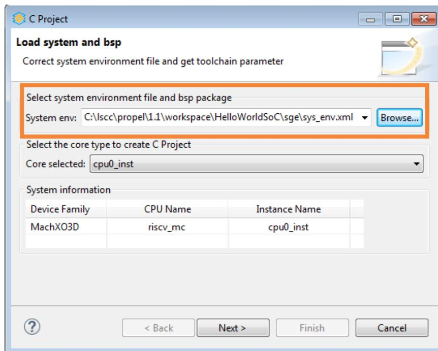
Figure 4.8. Load System and BSP Page
