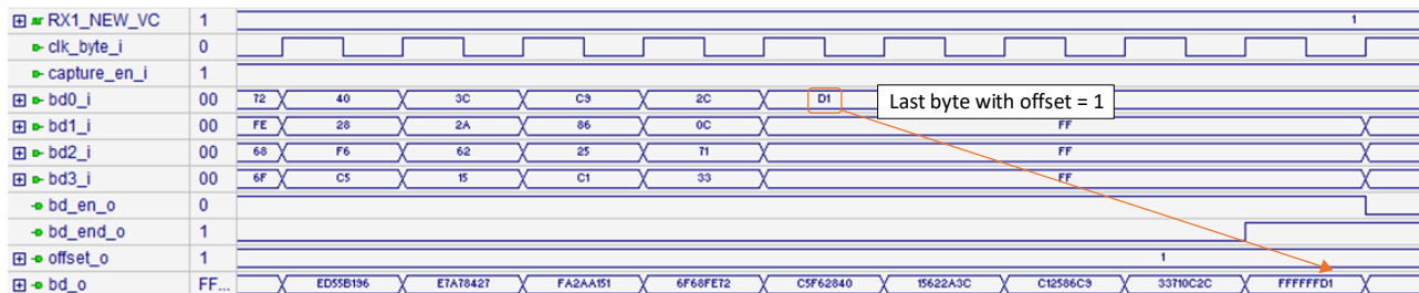
Figure 3.4. End of Long Packet with Trailer Bytes
