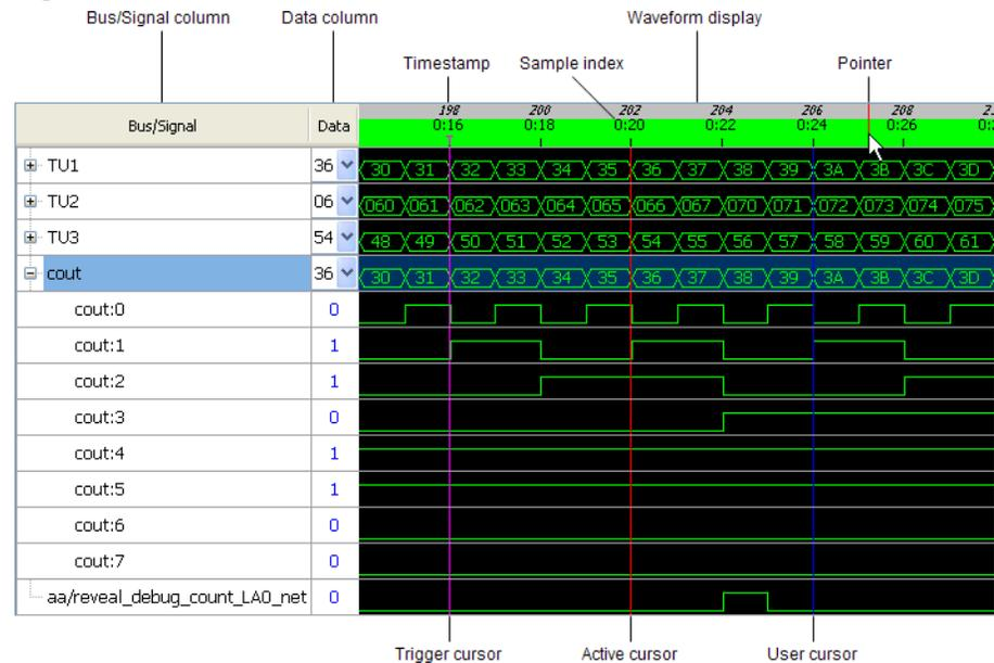
**Bus/Signal Column** Displays the names of the trace buses and signals in the selected module.
