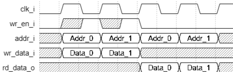
Figure 2.19. Distributed Single Port RAM Timing Waveform, Without Output Registers
