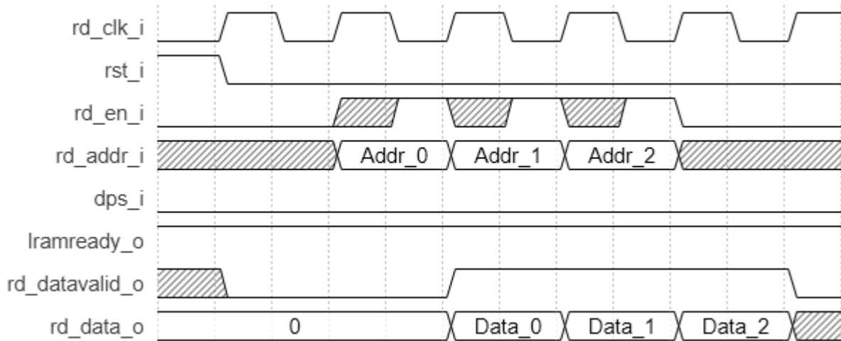
Figure 2.52. Large ROM Timing Diagram, Without Output Registers
