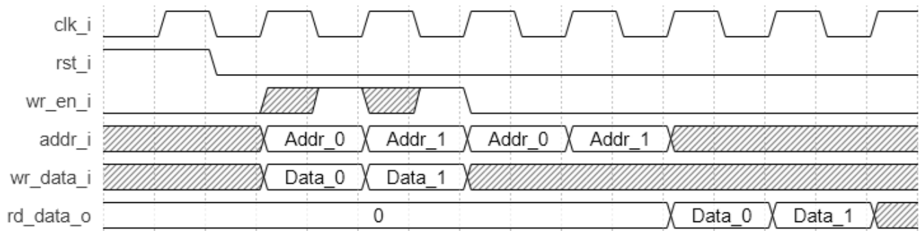
Figure 2.3. Single Port RAM Timing Waveform in Normal (NORMAL) Mode, With Output Registers
