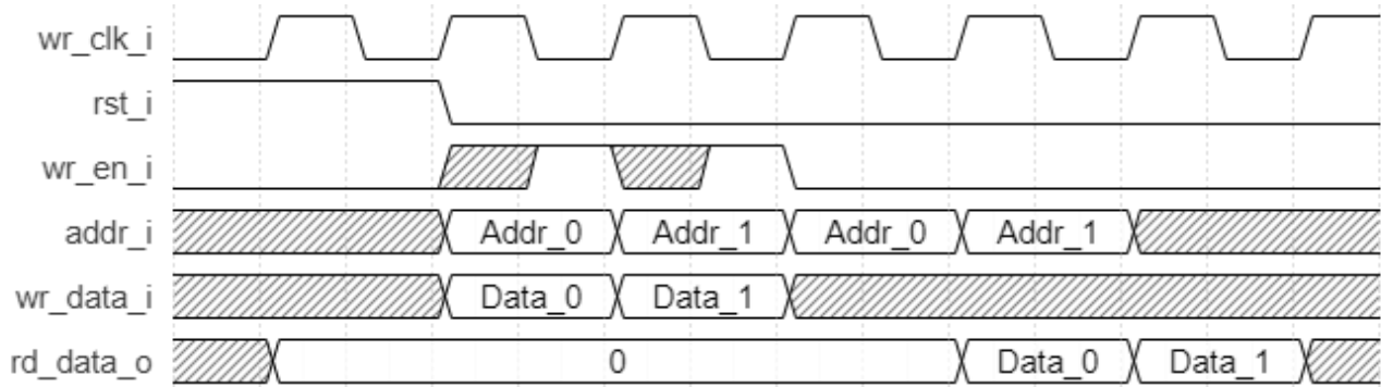
Figure 2.20. Distributed Single Port RAM Timing Waveform, With Output Registers and Synchronous Reset
