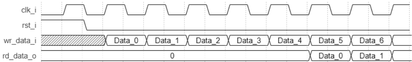
Figure 2.34. Shift Register Without Output Register
