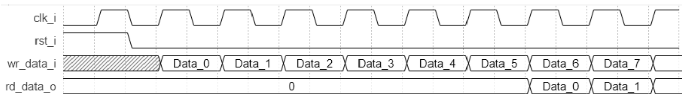
Figure 2.35. Shift Register With Output Register
