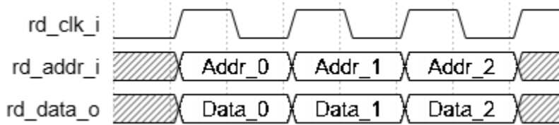
Figure 2.22. Distributed ROM Timing Diagram, Without Output Registers
