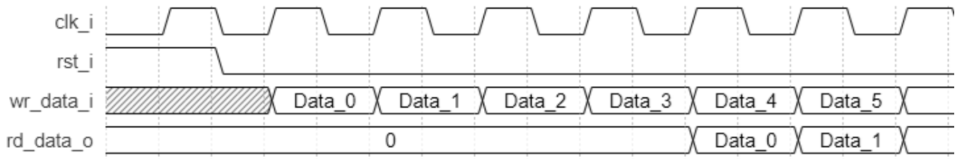
Figure 2.37. Shift Register Without Output Register (LUT Memory, Lattice Nexus Devices)
