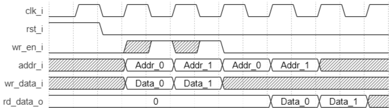
Figure 2.2. Single Port RAM Timing Waveform in Normal (NORMAL) Mode, Without Output Registers
