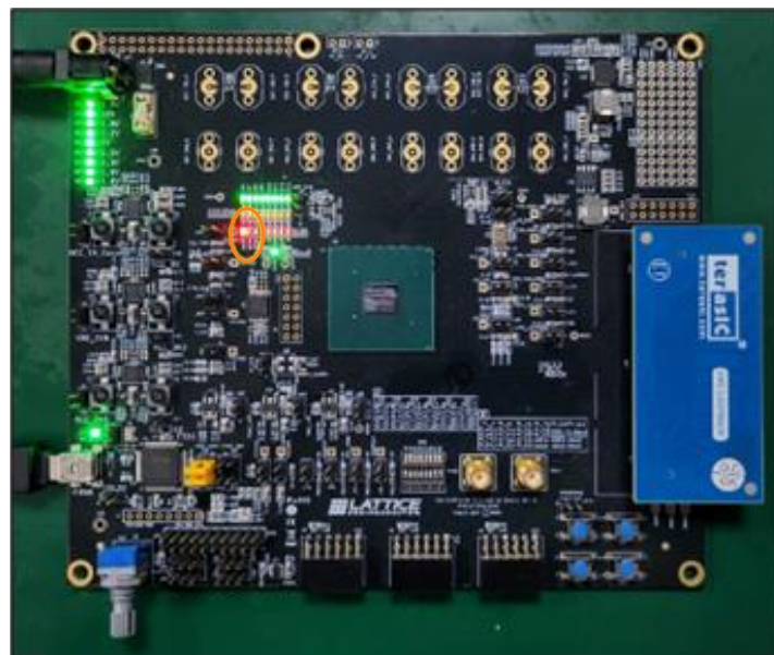
Figure 6.11. CertusPro-NX Evaluation Board with FMC Loopback Card on FMC Connector (J48)
