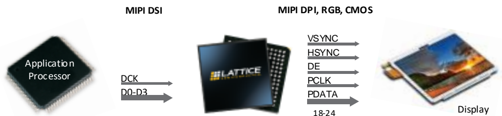
Figure 1.1. MIPI DSI to CMOS Interface Bridge IP System Diagram
