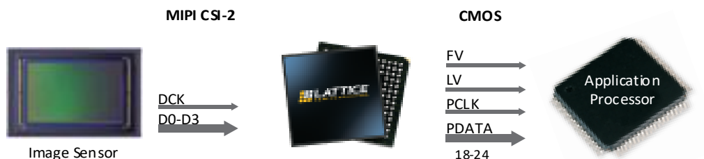
Figure 1.2. MIPI CSI-2 to CMOS Interface Bridge IP System Diagram
