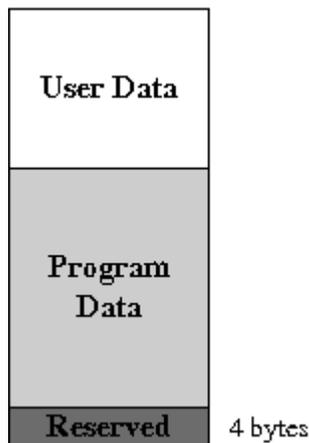
The scratchpad memory can be configured to be entirely internal to the LatticeMico8 microcontroller, entirely external to LatticeMico8 microcontroller, or a combination of both.
