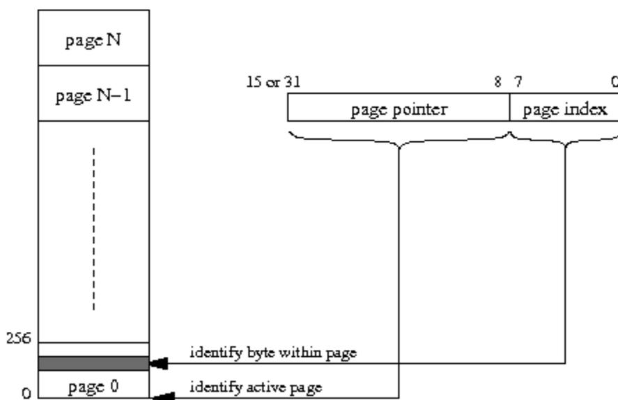
The page pointers are essentially general-purpose registers that have been retargeted to provide a memory address. (See [“Memory Regions” on page 5.](#)) Table 5 shows the memory modes of the LatticeMico8 microcontroller, the size of addressable memory space in each mode, and the general-purpose registers used as page pointers.
