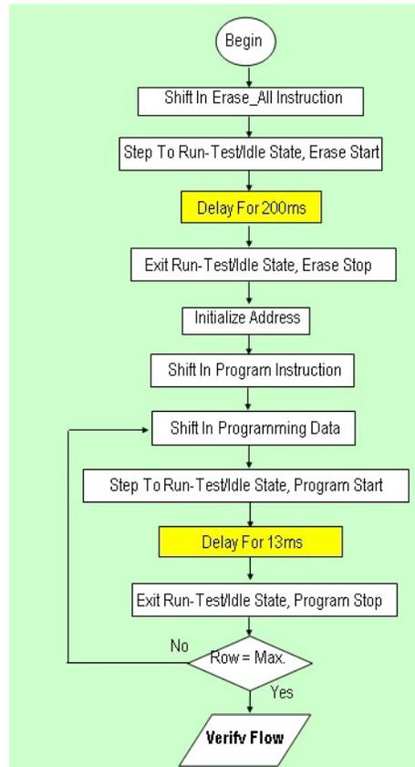
looping programming flow. The most critical requirement to ensure the devices are programmed reliably rests on the accuracy of the delay function.
