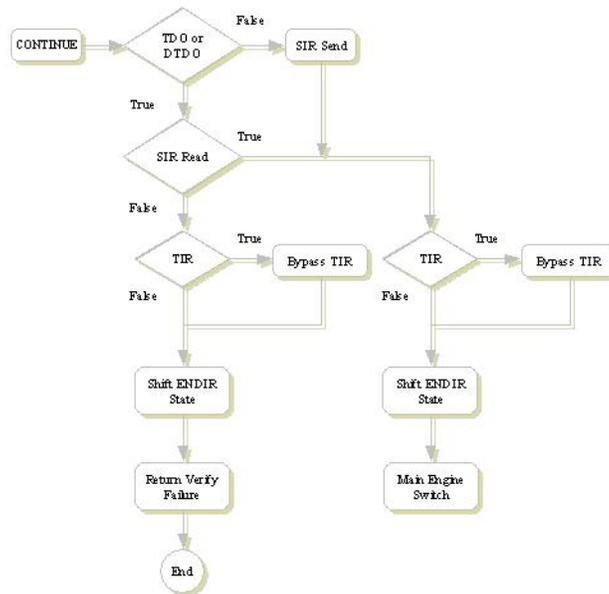
If the TDO or DTDO byte code were encountered in the SIR sub-switch, then that indicates that the SIR instruction is going to read data from the device, else the SIR instruction is going to send data to the device.
