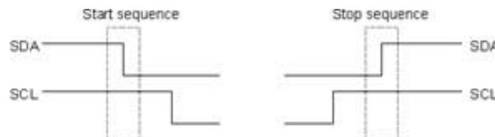
The primary I<sup>2</sup>C port of the Mach XO2 device can be used as a user I<sup>2</sup>C port function or as a device programming port. When used for device programming, the primary I<sup>2</sup>C port is a slave I<sup>2</sup>C with a default slave address
