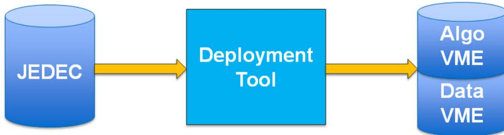
The programming data and programming instructions are compiled into a binary VME file format for the driver to load into the target devices. The VME file can be provided to the driver as a stand-alone file or linked together with the driver.
