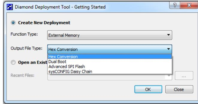
**Advanced** This operation is for generating hex files which handles more complicated operations such as Multiple Boot, and Quad I/O to configure external memory. Users can set the output hex format, how big the SPI Flash size is, whether or not to do a byte wide bit mirror, retain the bitstream header, and Whether or not to optimize the memory space. Another option is to set multiple user data file and where each of those data file's starting address should be in memory.
