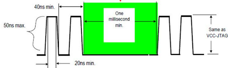
initialized to 0. If it is initialized to 1, then the TCK frequency is effectively reduced by half. Use this technique to reduce the TCK frequency until meeting the specification.
