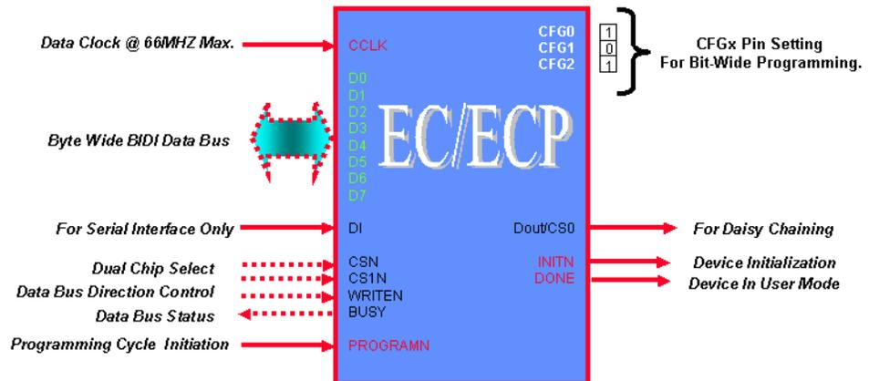
Only four pins, PROGRAMN, INITN, DONE, and CCLK, are dedicated. The other pins are dual purpose pins. Only the DI pin and DOUT/CS0 pin are used on serial programming.
