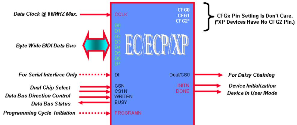
Only four pins, PROGRAMN, INITN, DONE, and CCLK, are dedicated. The other pins are dual purpose pins. The read back is turned on by selecting the Persistent On option when generating the bitstream.
