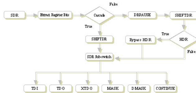
If CASCADE has not been set, then the processor shifts the device into the safe state DRPAUSE, and then to SHIFTR. If HDR exists (see HDR Case Statement), then the processor will bypass the HDR. The SDR sub-switch is a switch that is based off the byte codes that can potentially be found after the SDR byte code.
