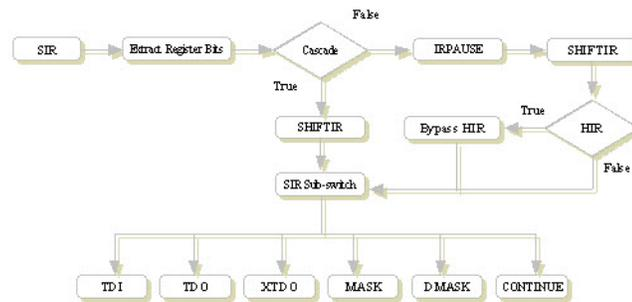
The TDO byte code indicates that there is data that needs to be read and verified from the device. The data following the TDO byte will be extracted and decompressed, if compression were selected, and held in memory until it is ready to be compared against data in the device.
