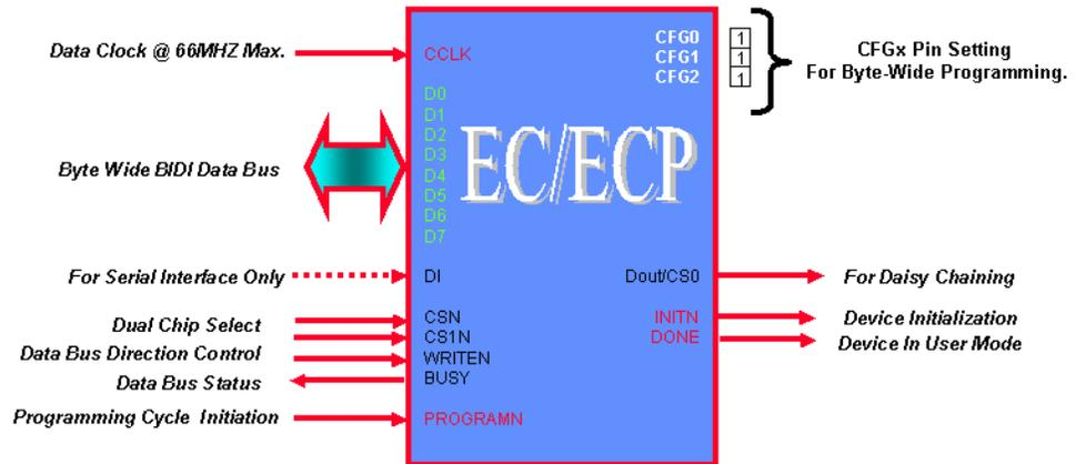
Only four pins, PROGRAMN, INITN, DONE, and CCLK, are dedicated. The other pins are dual purpose pins. The DI pin has no function on parallel programming.
