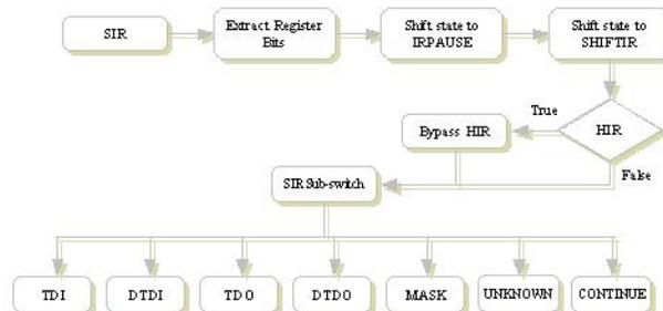
The SIR case statement begins by extracting the size of the register. The size will be used later to indicate how many bits of data will be sent or read back from the device. The processor then shifts the device into the safe state IRPAUSE, and then to the state SHIFTIR. If HIR exists (see HIR Case Statement), then the processor will bypass the HIR. The SIR sub-switch is a switch that is based off of the byte codes that can potentially be found after the SIR byte code.
