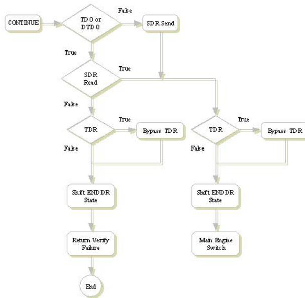
If the TDO or DTDO byte code were encountered in the SDR sub-switch, then that indicates that the SDR instruction is going to read data from the device, else the SDR instruction is going to send data to the device.
