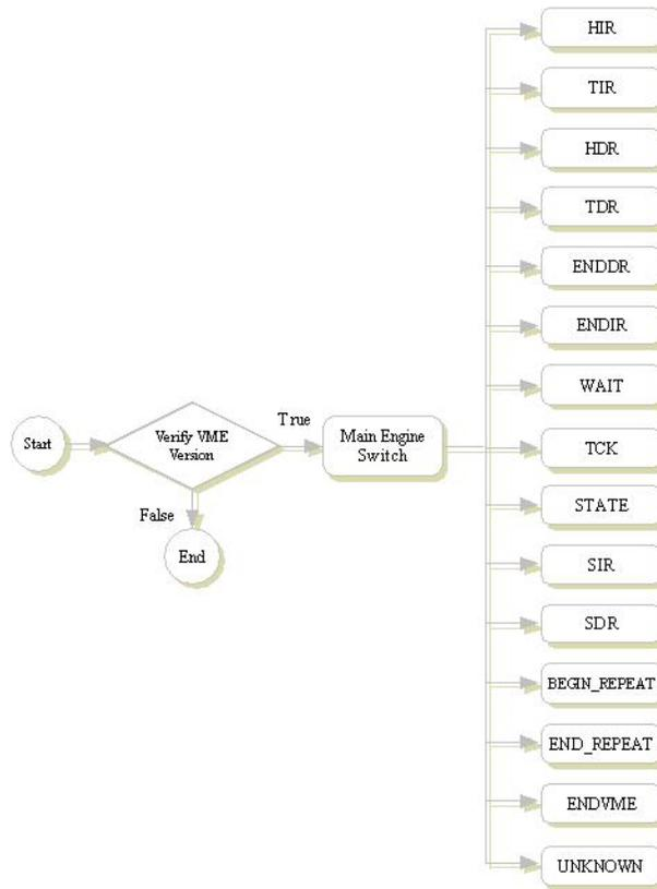
The Main Engine Switch calls the appropriate case statements based on the incoming byte code from the VME Algorithm buffer. Unrecognized byte codes will trigger the UNKNOWN case statement.
