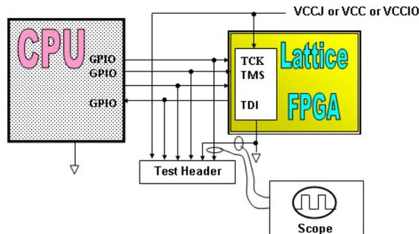
The calibrate function in Embedded VME can be launched by using the `-c` switch to cause the waveform as follow captured on the scope with the probe attached to the TCK wire.
