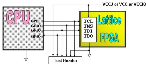
The pin mapping index table on the hardware.c must be revised to match with the customer's board layout. On the PCB that is the target for porting the Embedded VME, it is important and a good practice to route the JTAG port to a test header for easy access using an oscilloscope or connecting to Programmer for debugging.
