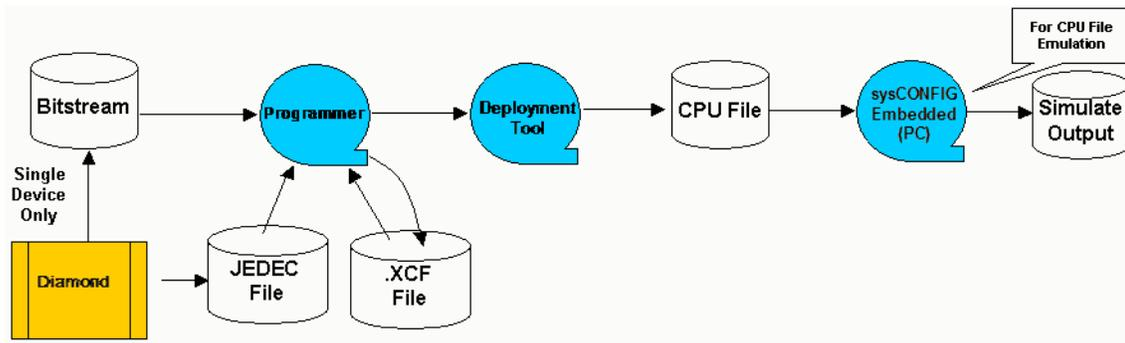
**sysCONFIG Embedded Bitstream Generation** You can use Deployment Tool to generate sysCONFIG Embedded bitstreams for the current Lattice FPGA device chain.
