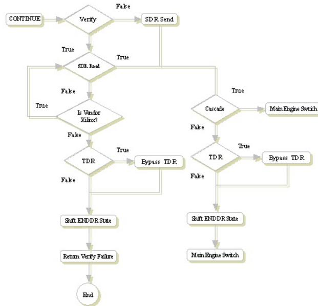
If the TDO or XTDO byte code were encountered in the SDR sub-switch, then that indicates that the SDR instruction is going to read data from the device, else the SDR instruction is going to send data to the device.
