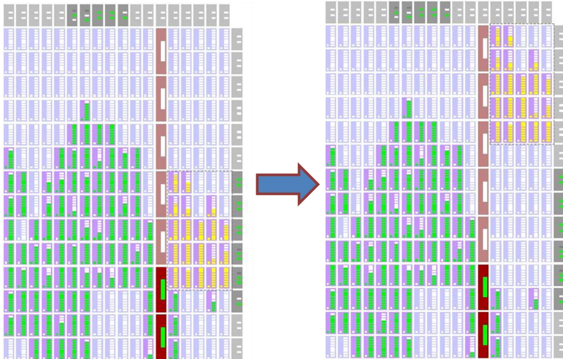
Figure 7-13: Moving a group of Logic Cells
