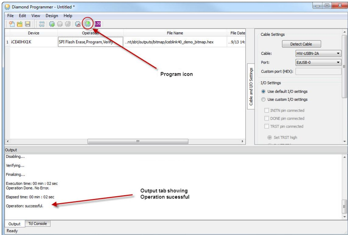
**Figure 24: Diamond Programmer Main Window – Successful Program Operation**
