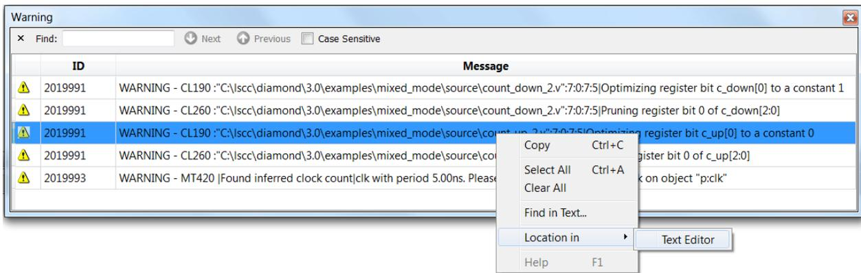
The Error, Warning, and Info views can be selected, closed, opened, detached, and attached using the double-click method. See “Basic UI Controls” on page 27.
