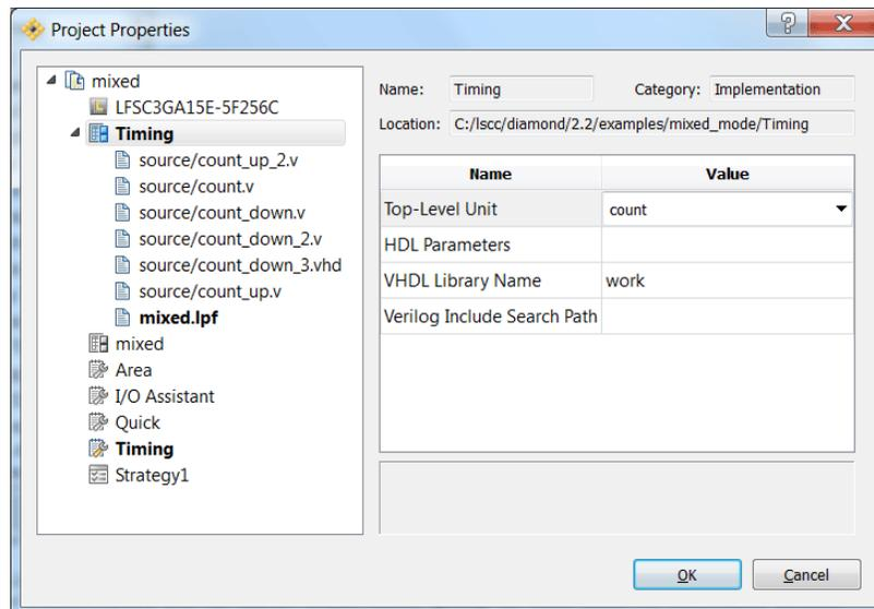
In the Project Properties dialog box, select **Value** next to **Top-Level Unit** and select the desired top level from the list.
