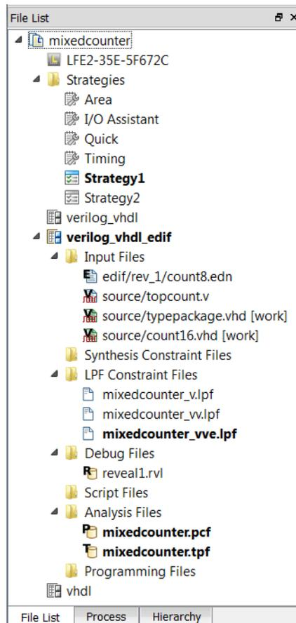
After you add a module, use the **Include For** menu to specify how the module file is to be used in the design.
