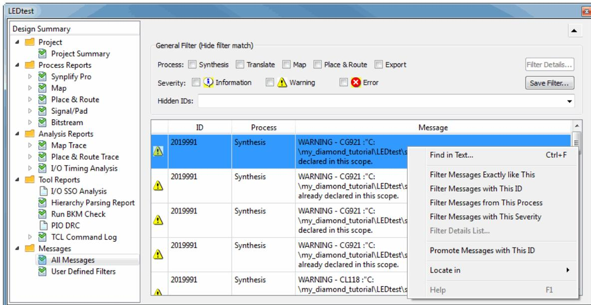
When you save a message filter, its name appears in the Messages section of the Design Summary pane under “User Design Filters.” When you select the filter, all the filtered messages are hidden in the report pane. When you re-select All Messages, the filtered messages are again displayed.
