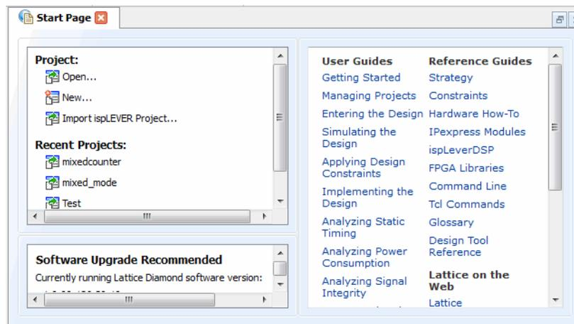
The Start Page can be closed, opened, detached, and attached with the Attach button. See “Basic UI Controls” on page 27.
