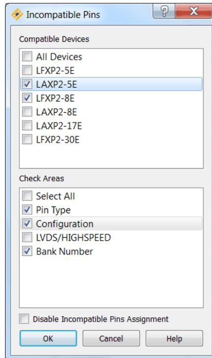
The “Incompatible Pins” dialog box is available from the View menu in Spreadsheet View or Package View after the Translate Design process. After selecting one or more devices for possible pin migration, you can view the incompatible pins in Package View and in the Pin Assignments sheet of Spreadsheet View.
