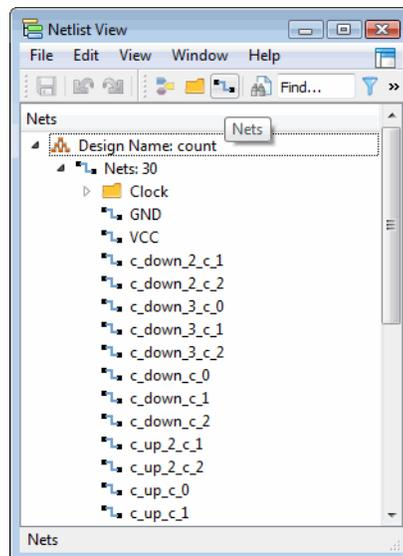
From Netlist View, you can drag selected signals to Package View to assign them, drag selected nets to Spreadsheet View's Route Priority sheet to prioritize them, and drag registers to the Cell Mapping sheet to specify registers for flip-flops. You can use the right-click menu to set timing preferences for selected nets and to create logical groups from selected instances.
