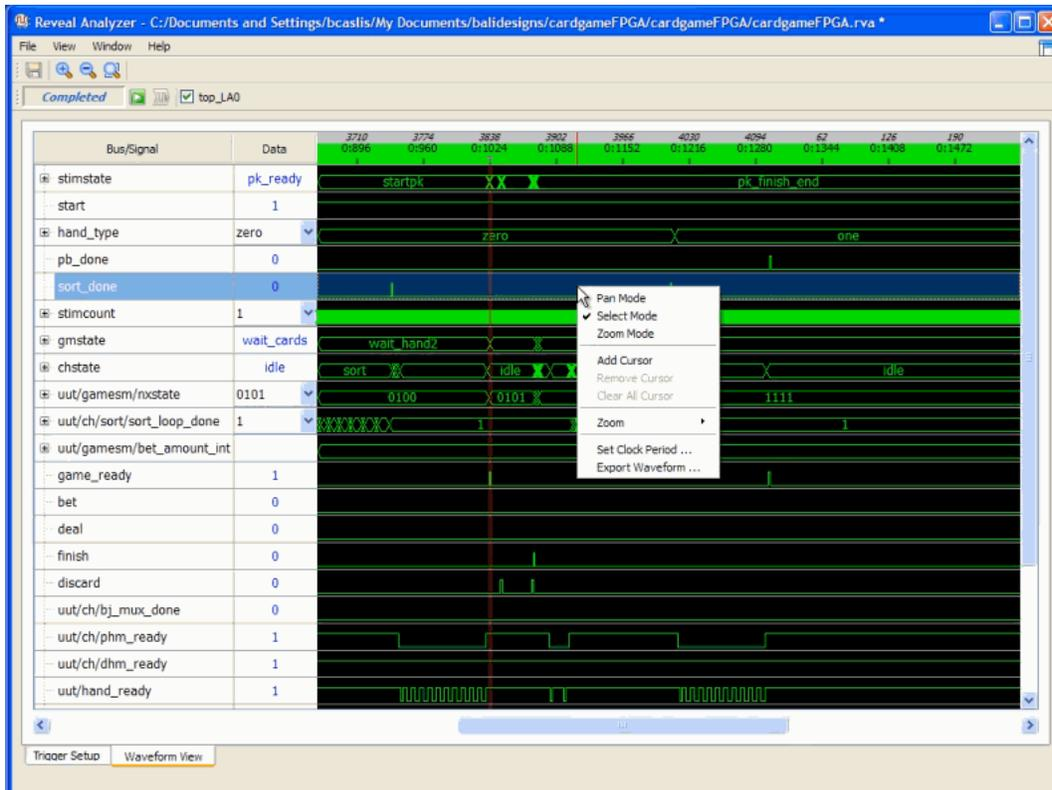
The Data column in the view shows the data for the active cursor. The Reveal Analyzer supports multiple cursors which can be added, removed and position changed within the waveform. Selecting the cursor and dragging it will produce a rubber band effect which can be used for measuring time intervals.
