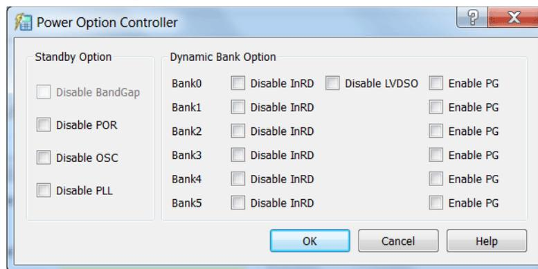
First, set the standby, shut-off, and power guard options that you want to allow, using the appropriate Power Calculator pages. Afterwards, return to the Power Summary page, click the **Power Control** button to open the Power Option Controller, and select the elements to be turned off during low-power operation.
