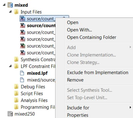
You can use the “Include for” commands to specify that a source file be included for both synthesis and simulation, synthesis only, or simulation only.
