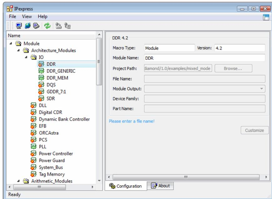
In addition to the included modules, an IP Server button is provided that enables you to connect to the Lattice IP server, explore the available IP, and select those that you would like to download and install. In Diamond 2.1, IPexpress indicates whether an IP from the IP server is compatible with the running software release. The three states are compatible, incompatible, or unsupported.
