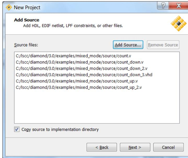
This process of browsing and adding source files can be done as many times as needed before going to the next step.
