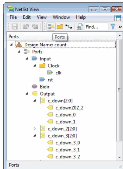
Each design tree view is equipped with utilities for filtering the list and searching for elements.
