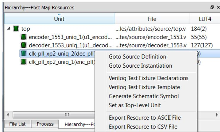
After synthesis, the Hierarchy view displays the calculated resource utilization data, such as LUT4, registers, and I/O registers. Device resources that would be consumed are shown to the right of each module. The first number in each column indicates the quantity of that resource that would be used by that module and all of its submodules. The second number, in parentheses, indicates the quantity of that resource that would be used by just that module, not including any of its submodules.
