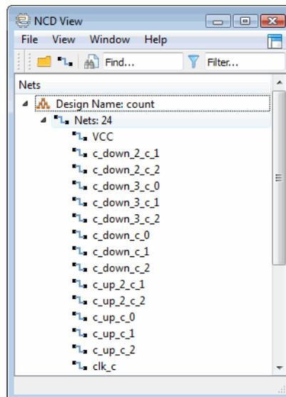
Each design tree view is equipped with utilities for filtering the list and searching for elements.
