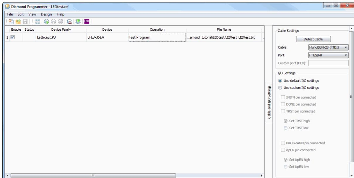
Programmer supports serial, concurrent (turbo), and microprocessor programming of Lattice devices in PC and Linux environments. Device chains can be scanned automatically using the Programmer graphical user interface.
