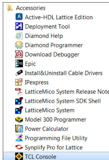
Select this Tcl Console to run the external Tcl shell. You can enter “help” at the prompt to see the major groups of Tcl commands for Lattice Diamond. Help on individual commands is available both in the online Help and from the “help” command within the console. The console’s help command can be used to get the top level help, help for a particular dictionary, or help for an individual command.
