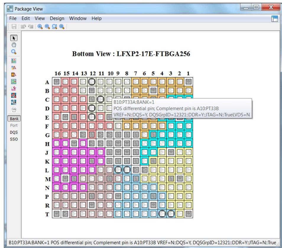
As you move your mouse pointer over the layout, pin descriptions and locations are displayed in tool tips and in the status bar. The **View > Show Differential Pairs** command displays fly wires between differential pin pairs and identifies the positive differential pins.
