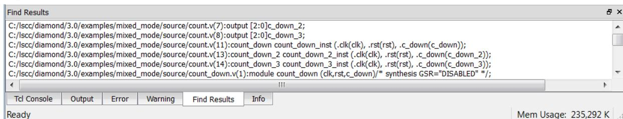
The Find Results view can be selected, closed, opened, detached, and attached using the double-click method. See “Basic UI Controls” on page 27.
