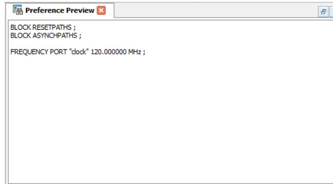
The Preference Preview is a read-only view of logical preferences and can be opened, closed, detached and attached (using the attach button).
