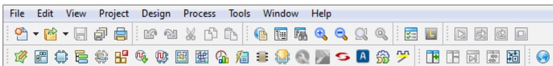
The toolbars are organized into functional sets. The display of each toolbar is controlled in the **View > Toolbars** menu and also by right-clicking in the Menu and Toolbar area. Each toolbar can be repositioned by dragging and dropping it to a new location.
