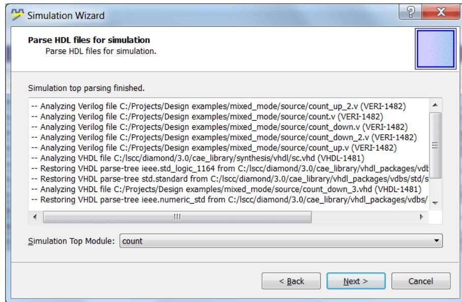
In some designs, the compile order of the HDL files passed to the simulator might result in compilation warnings. In most cases, these compilation warnings can be safely ignored. The warnings can be eliminated in one of two ways:
