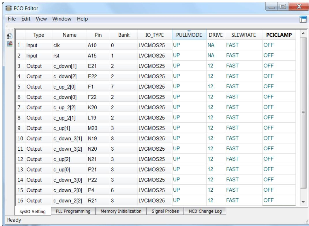
ECOs are requests for small changes to be made to your design after it has been placed and routed. The changes are directly written into the native circuit description database file (.ncd) without requiring that you go through the entire design implementation process.
