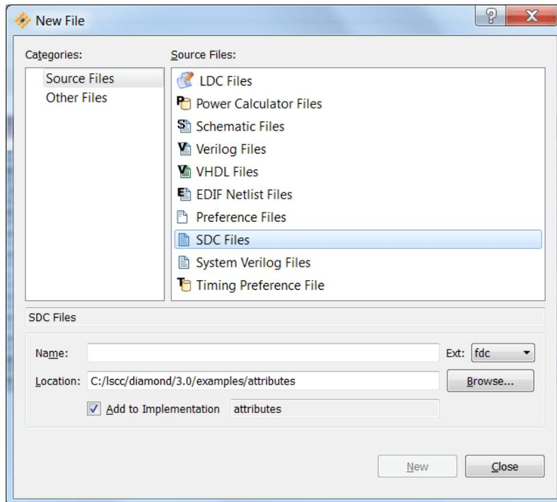
If you selected SDC Files, open the file in the Source Editor to add the constraints. If you selected LDC Constraint Files, the LDC Editor will open displaying the spreadsheet and six tabs for creating and editing synthesis constraints.
