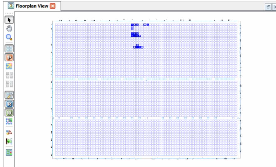
Floorplan View allows you to create REGIONS and bounding boxes for UGROUPs and specify the types of components and connections to be displayed. As you move your mouse pointer over the floorplan layout, details are displayed in tooltips and in the status bar:
