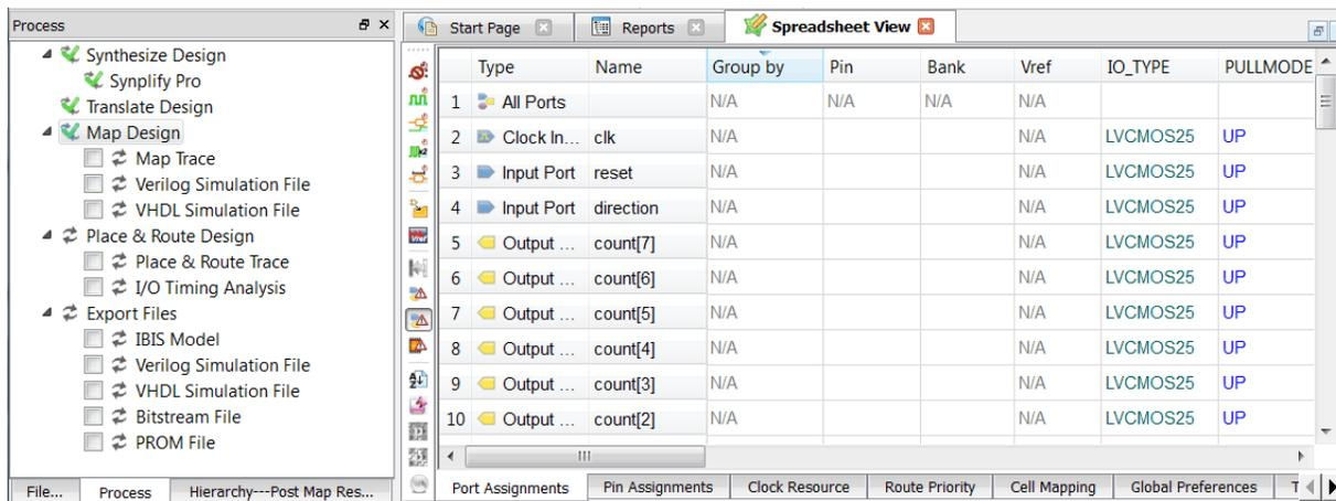
After Place & Route Design has been completed, Spreadsheet View displays the pin assignments.
