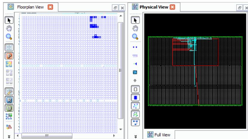
When you right-click the selected signal in Physical View and choose **Show In > Floorplan View**, the same selected signal is highlighted on the Floorplan View layout, as shown in Figure 23.
