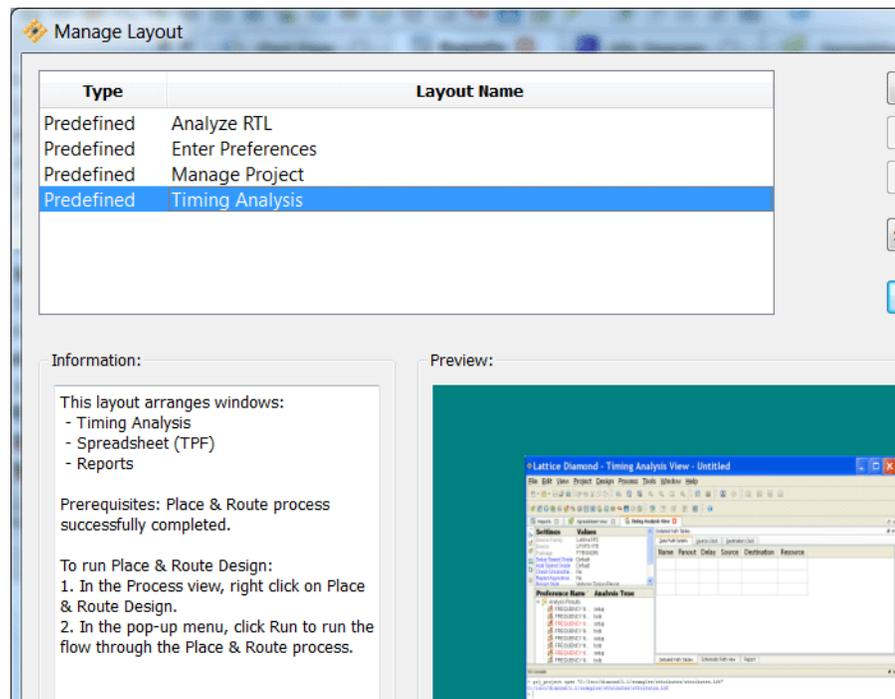
provides prerequisites and instructions for viewing all the windows of the layout. For example, if you load the Timing Analysis predefined layout and your design is still in the pre-route stage, you will need to run Place & Route in order to view the Timing Analysis View.
