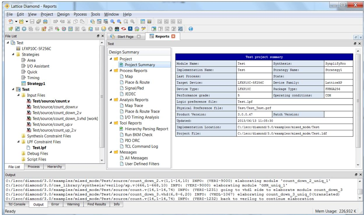
Select the **File List** tab under the left pane, to view the Test project file list. Select the **Process** tab, to view the design flow processes and status.
