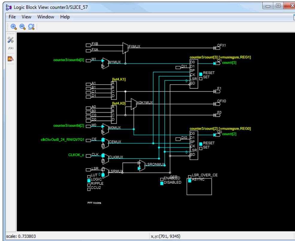
Schematic views of PIO and PFU/PFF components can be accessed from NCD View, Floorplan View, and Physical View. Tabular views of PLL, EBR, and DSP blocks can be accessed from Floorplan View and Physical View. Right-click one or more selected components and choose **Logic Block View**.
