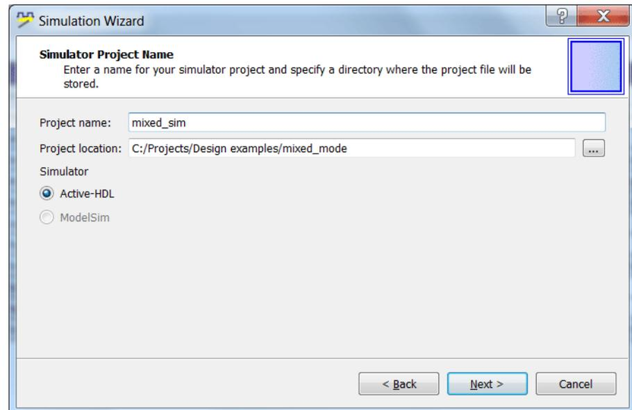
After you have set up the simulator project and specified the implementation stage and source files to be included, the Simulation Wizard parses the HDL and test bench. The last step is to specify the simulation top module.
