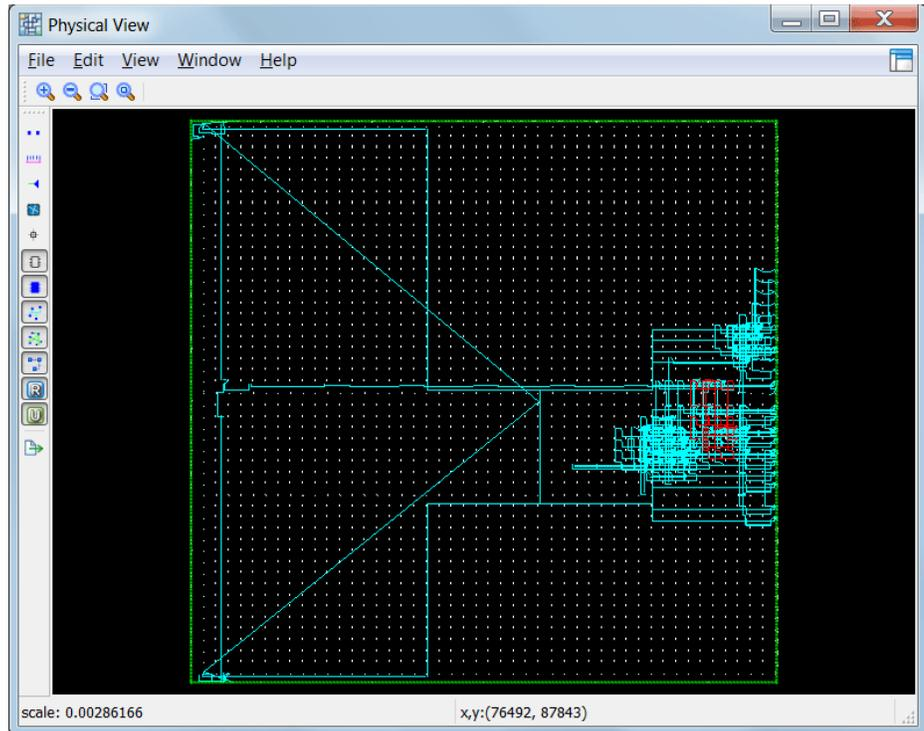
As you move your mouse pointer slowly over the layout, the name and location of each REGION, group, component, port, net, and site are displayed as tool tips and also appear in the status bar. The tool tips and status bar also display the group name for components that are members of a group.
