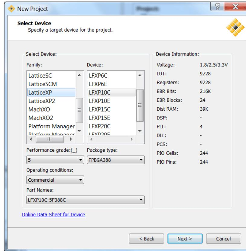
In this step you can select the target device, performance grade, package type, operating conditions and part name. For our example, we will use the default settings.
