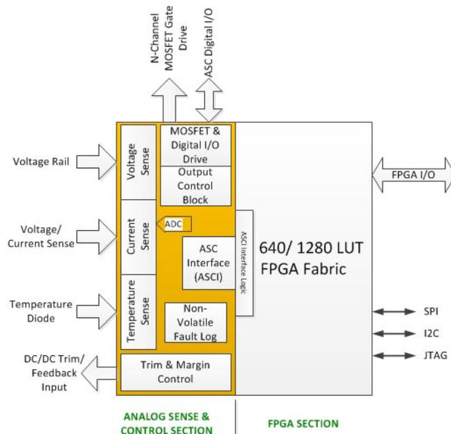
The Platform Manager 2 device is made up of an Analog Sense and Control block and an FPGA block. These two blocks provide the necessary programmable building blocks to enable integration of various combinations of hardware management functions into a single chip. The hardware
