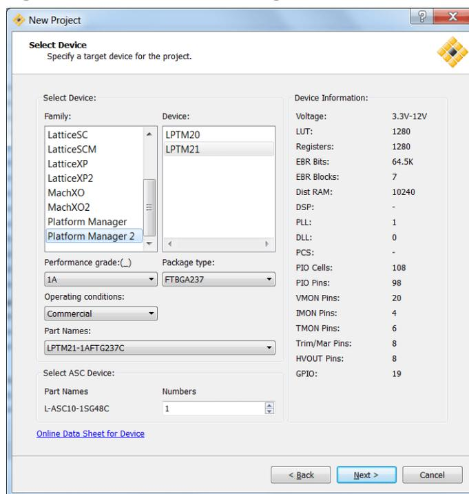
Platform Manager 2 devices contain one embedded Analog Sense and Control (ASC) device. The LPTM21 device allows you to add one external ASC device. The LPTM20 device does not include this option. To add an external ASC device, select **LPTM21**. The “Select ASC Device” section will then appear near the bottom of the dialog box.
