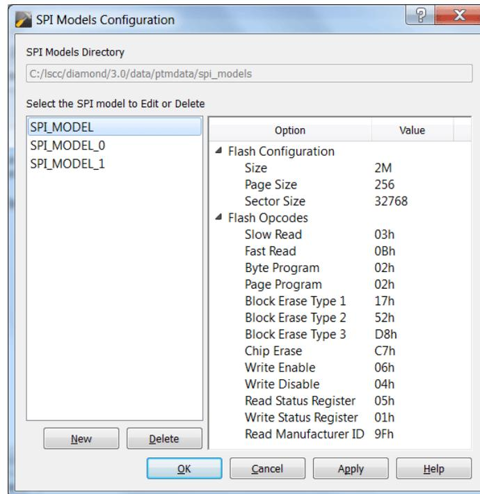
The SPI Models Configuration dialog box displays the library of currently available SPI models.
