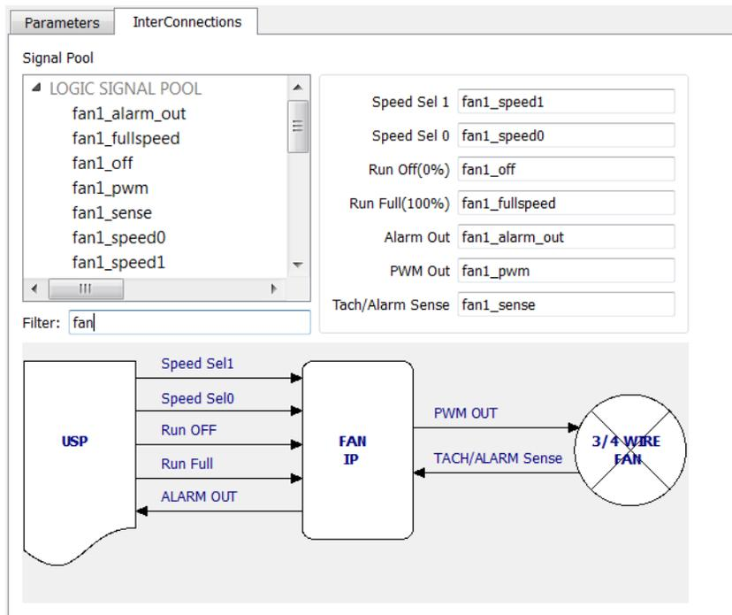
11. Drag the desired signals from the Signal Pool to set the logical connections for Speed Sel, Run Off, Run Full, and Alarm Out.
