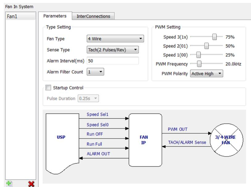
3. Select the Parameters tab and in the Type Setting section, select the fan type.
