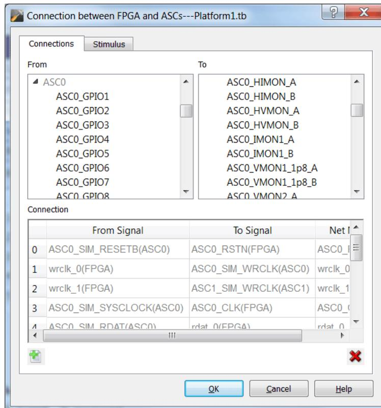
The “Connection” section, at the bottom, displays the default hardware connections between the FPGA and all ASC devices in the design. These cannot be edited or removed.
