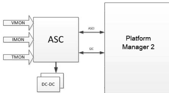
Multiple ASC devices (up to 8) can also be connected to a MachXO2 HC device (640 LUT or higher), similar to the Platform Manager 2, to offer wider flexibility and control when implementing a complete hardware management system as shown in Figure 3.
