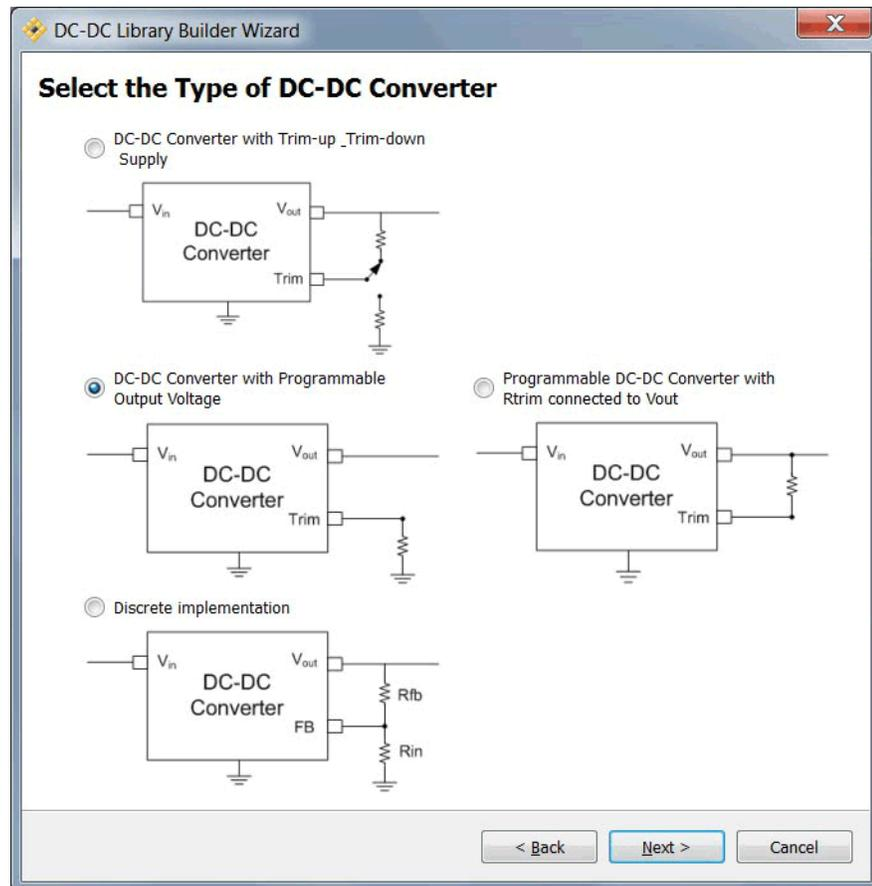
The wizard opens the Configuration portion of the dialog box, which enables you to set the parameters for the type of converter you selected.
