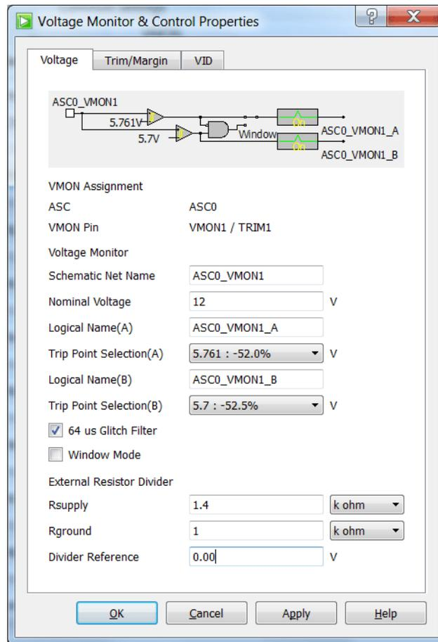
logical high if the Comparator B output is high and the Comparator A output is Low (i.e., the voltage monitor reading is between Comparator A and Comparator B).
