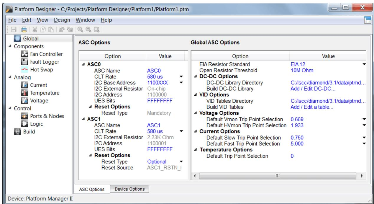
**Global** The **Global** Configuration view, provides global configuration options, including options for each ASC device. The global ASC Options provide access to dialog boxes that enable you to add a DC-DC converter to the DC-DC library and a voltage identification table to the VID library. The Device Options enable you to select the programming interface and clock source, set the boot mode, and configure SPI models.
