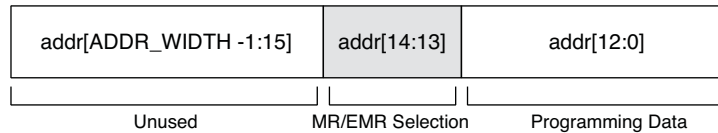
Figure 2-9. Local-to-Memory Address Mapping for MR/EMR Programming
