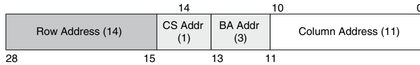
Figure 2-8. Mapped Address for the Example
