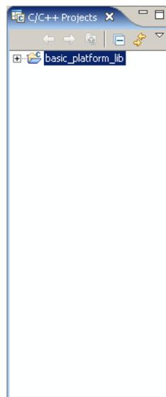
7. Select the `basic_platform_lib` project and build it by selecting **Project > Build Project**.
