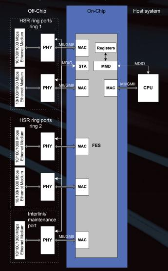
All of the ports of FES-HSR can be either copper or fiber Ethernet interfaces, or connected to other FPGA blocks. Packet forwarding takes place at wire-speed and the switching operation is non-blocking. These IP cores support the following interface options:
