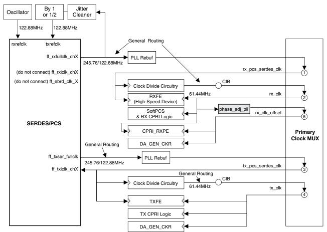
Figure 4. Clock Configuration for CPRI Slave Application
