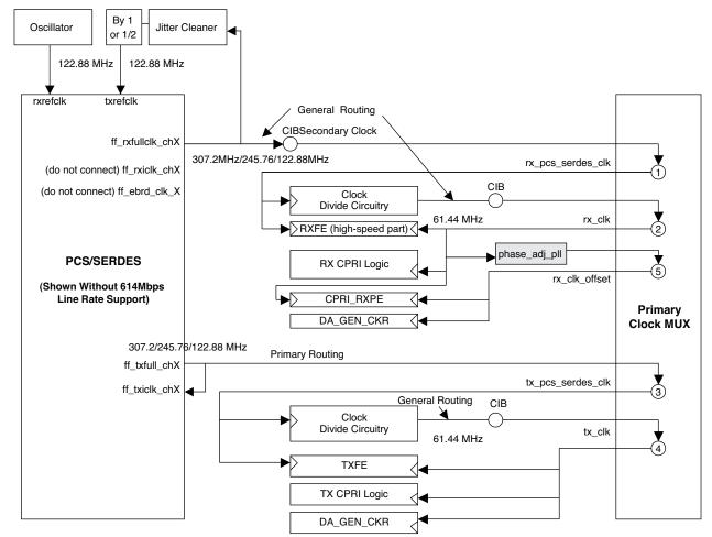
Figure 10. Clock Configuration for CPRI Slave Applications
