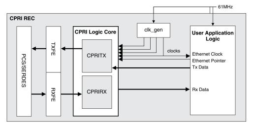
The CPRI IP logic core is provided in NGO format and is identical for both the basic and low latency core configurations. However, the RXFE and TXFE logic blocks and the SERDES/PCS configuration differ significantly for the low latency configuration versus the basic configuration.
