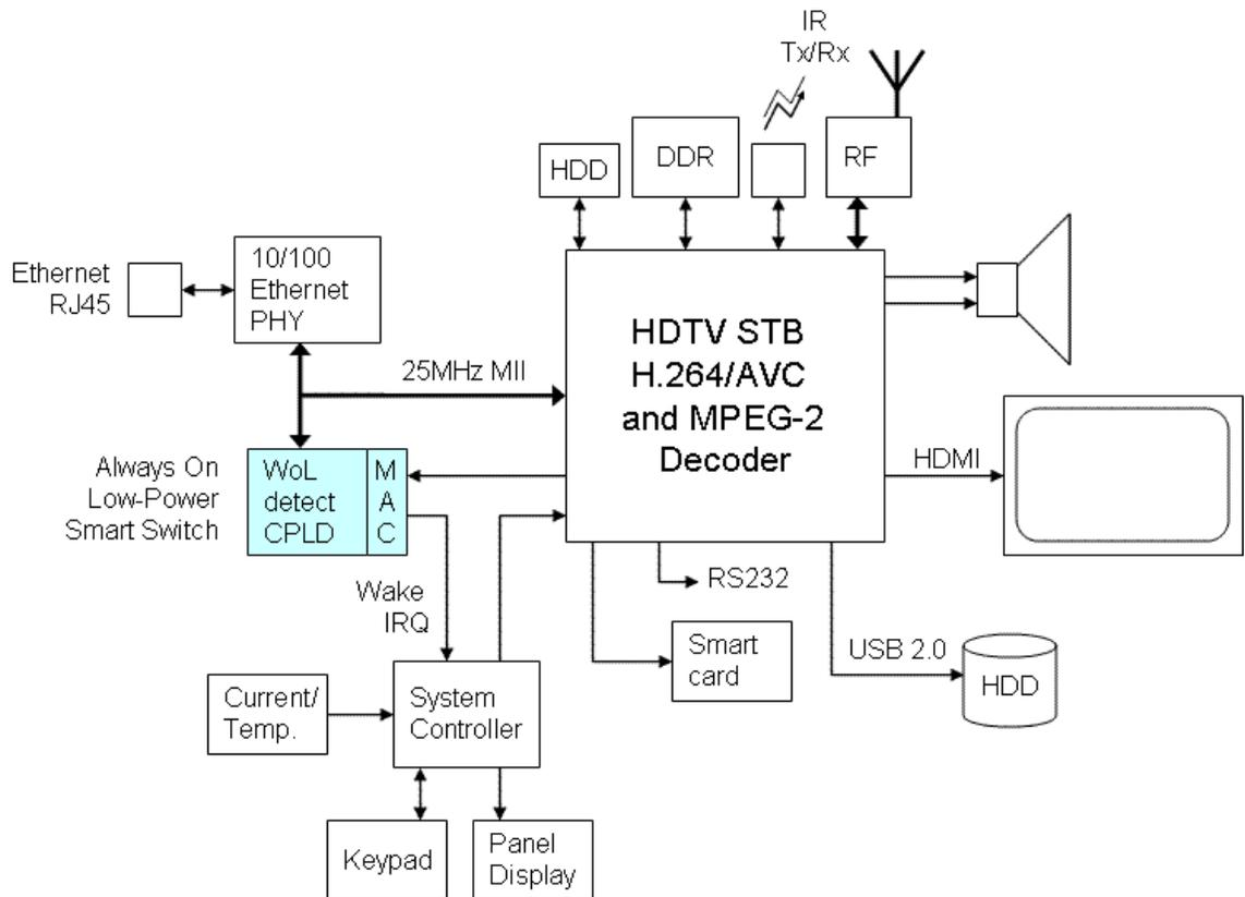
**Figure 1 - IP-TV STB with CPLD-based Smart Switch**
