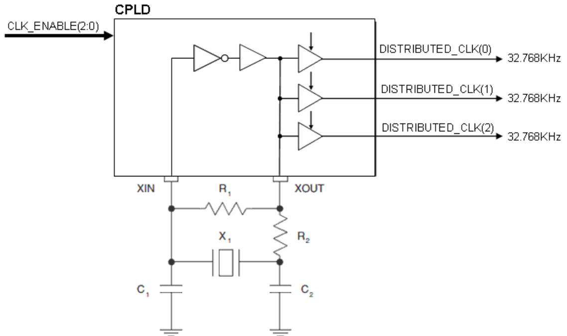
**Figure 2 - CPLD with Crystal Pierce Circuit**
