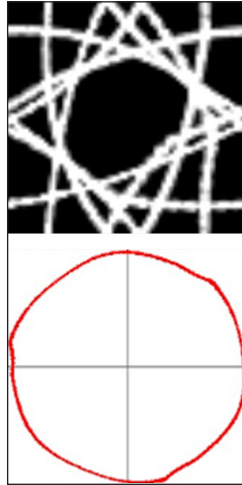
Figure 10: PDM Images of Motor with Balanced Currents and Load
