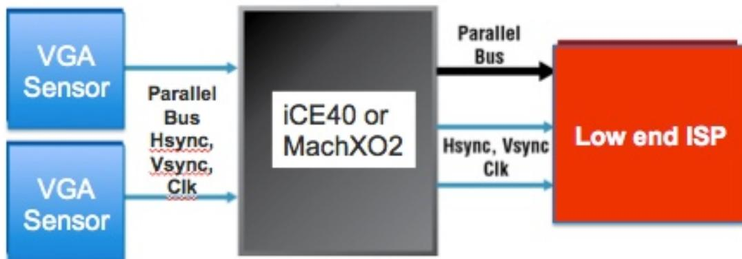
*Dual image sensor bridge using a MachX02 or iCE40 FPGA*
