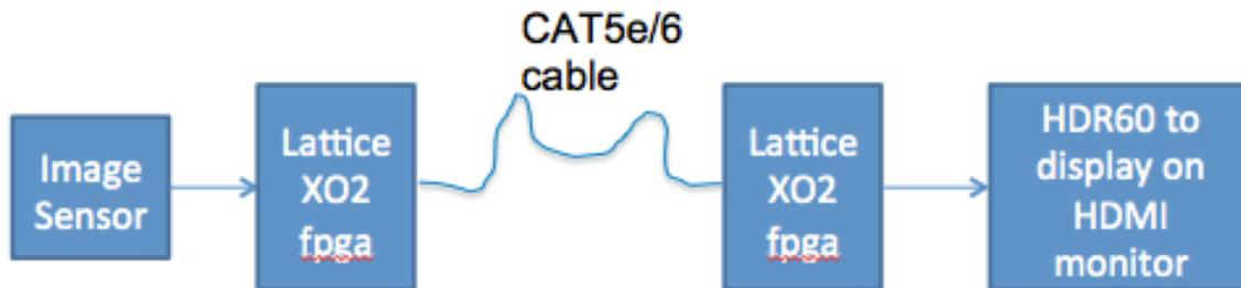
*Image sensor extender using two Lattice XO2 FPGAs and a Cat 5e/6 cable.*
