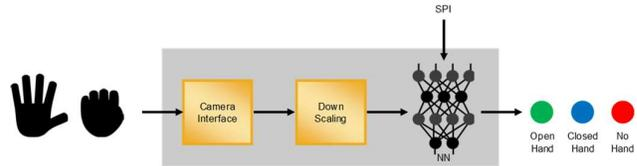
Figure 2: A system diagram for a low power gesture detection solution for use in Edge devices
