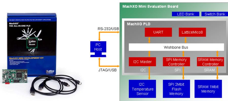
**Figure 4 - MachXO Mini Development Kit & evaluation board block diagram**
