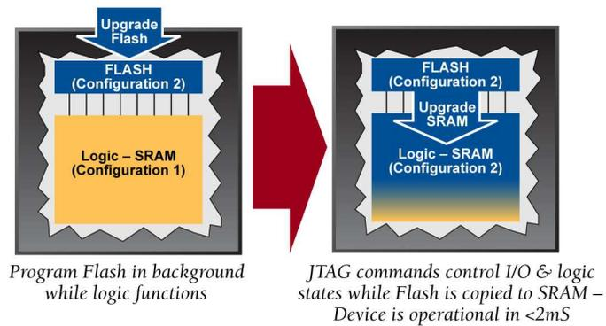
**Figure 3 - TransFR operation using MachXO PLDs**
