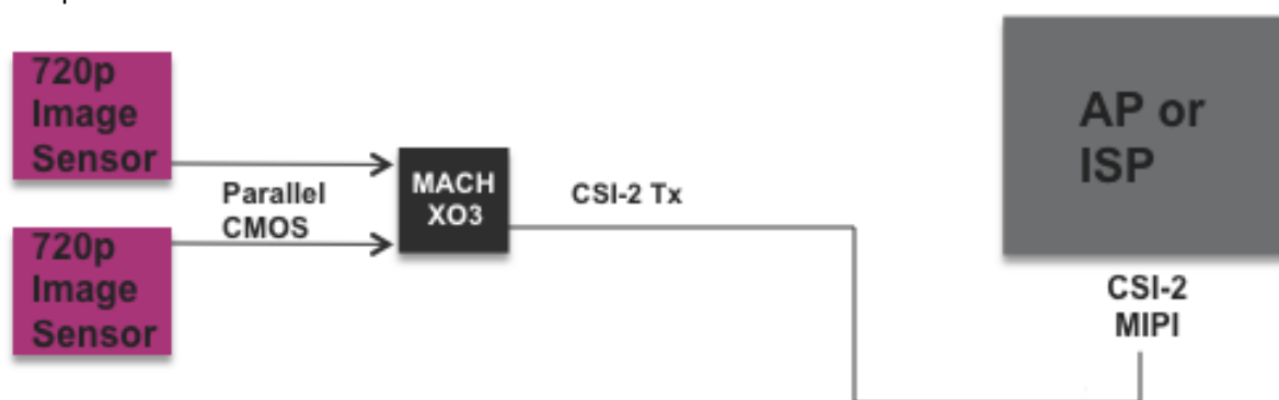
Figure 5: Dual sensor bridge expands existing system functionality.
