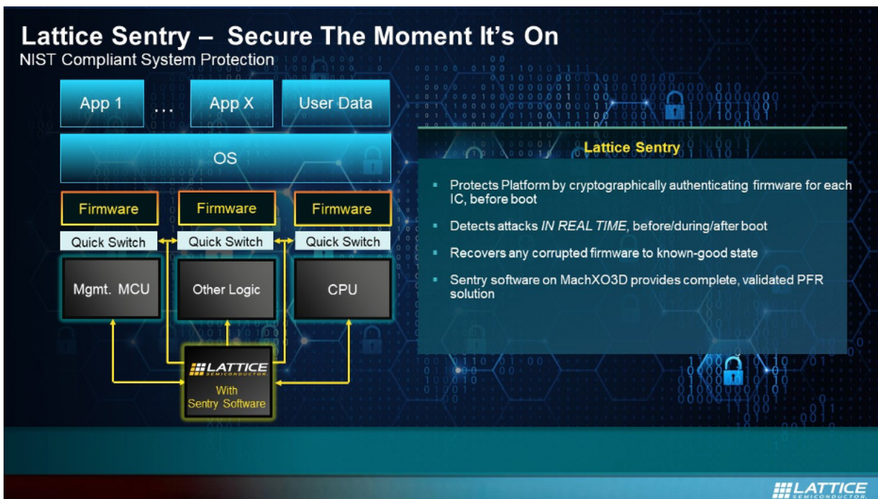
Figure 4: The block diagram illustrates how a Lattice Sentry-based PFR application can protect all firmware instances in a system in real time.
