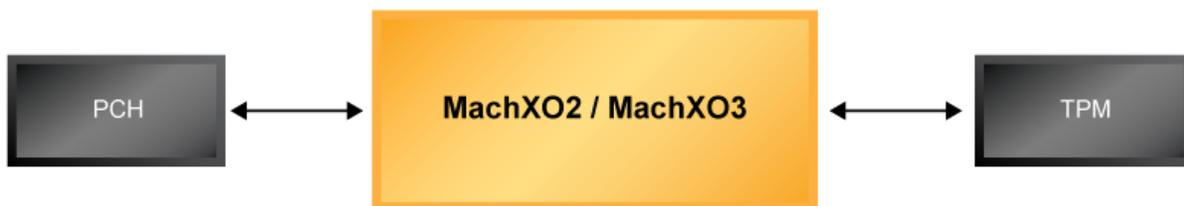
**Fig. 8: LPC to SPI Bridge for TCM.**
