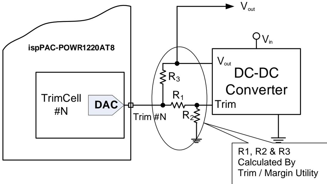
**Figure 9 – TrimCell Driving a DC-DC Converter**
