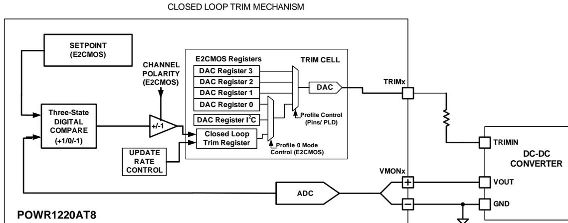
**Figure 6 – TrimCell Operating in Digital Closed Loop Trim Mode**
