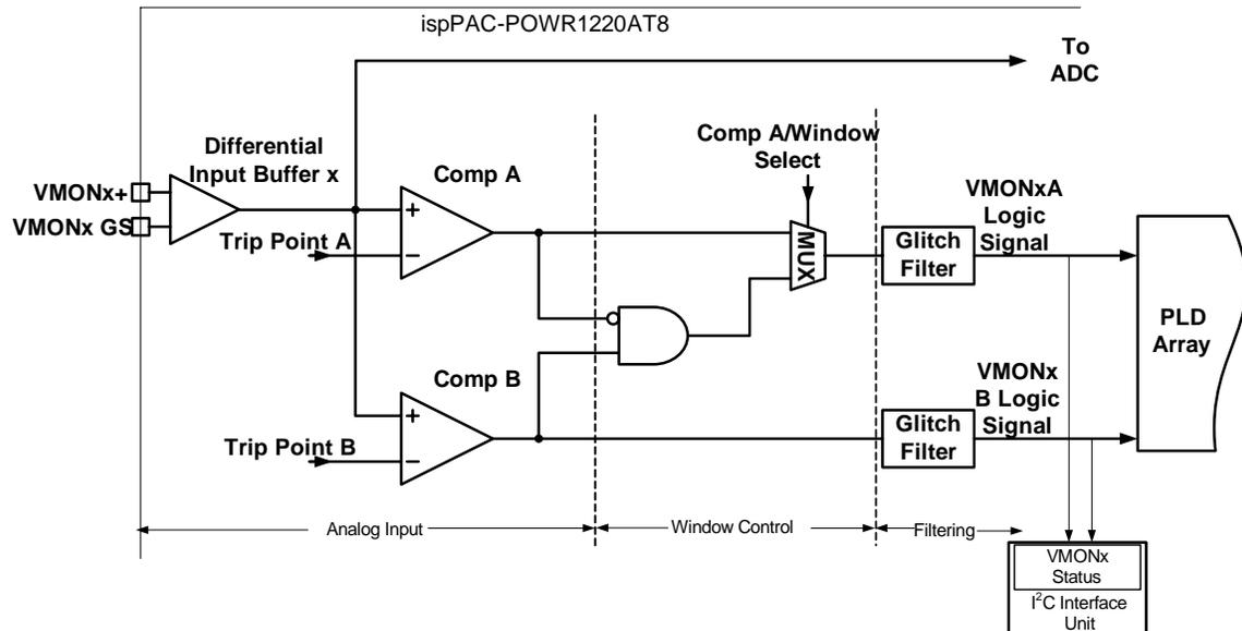
**Figure 2 - Architecture of Voltage Monitoring Input**
