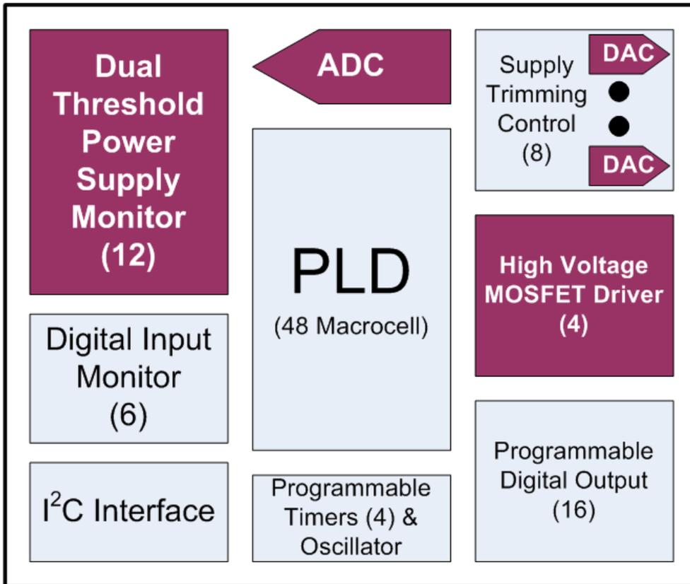
**Figure 1 – Power1220AT8 Block Diagram**
