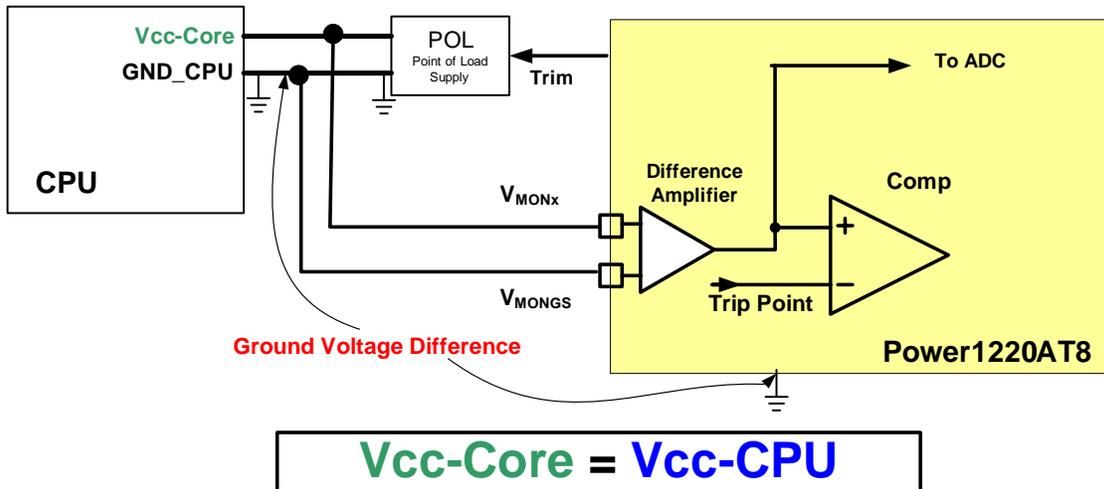
Ground Voltage Difference is the instantaneous Voltage difference between the GND\_CPU and Power Manager Ground
