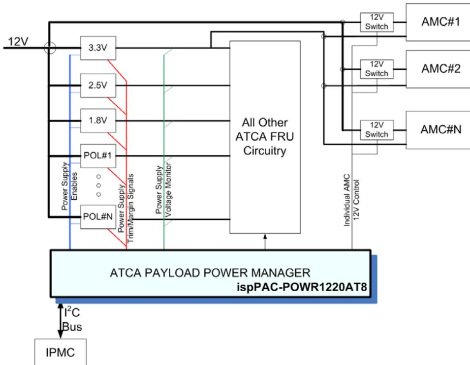
**Figure 7 - Power Management Circuit of an ATCA FRU**
