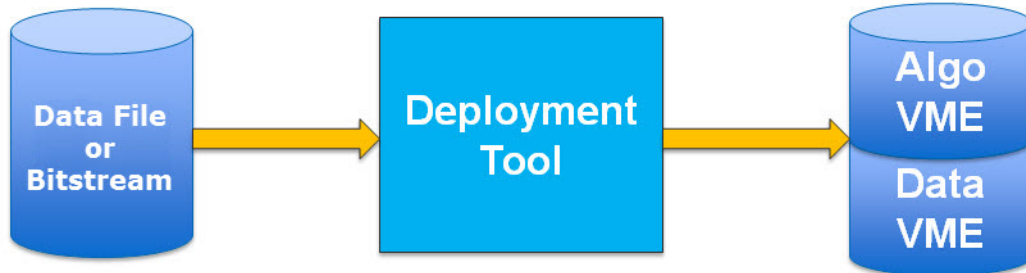
Figure 9: Full Embedded VME Flow
