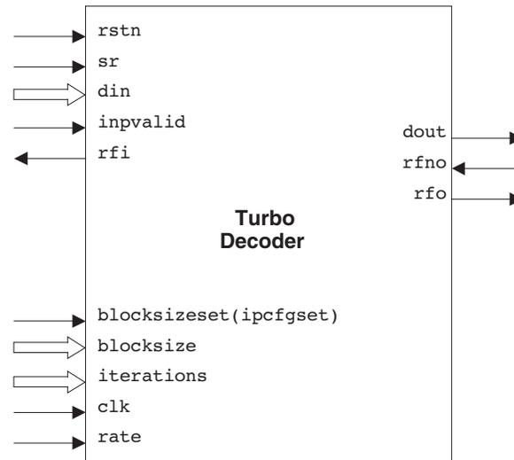
Note: Additional I/O signals are required if either an external memory or double buffer is selected. Please refer to the Additional Signals for External Memory section of this document for further information.
