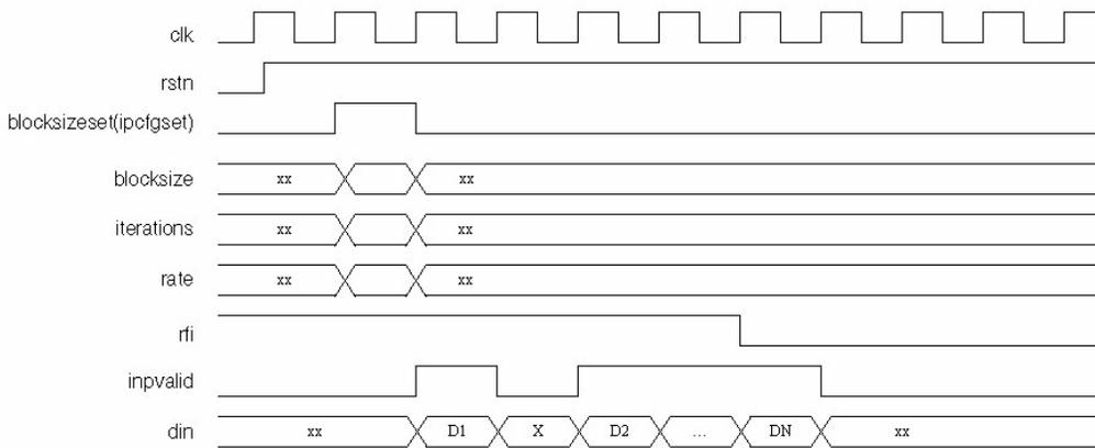
Note: Signals are transferred on the rising edge. N is the block size.
