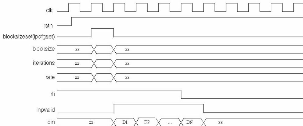
Note: Signals are transferred on the rising edge. N is the block size.
