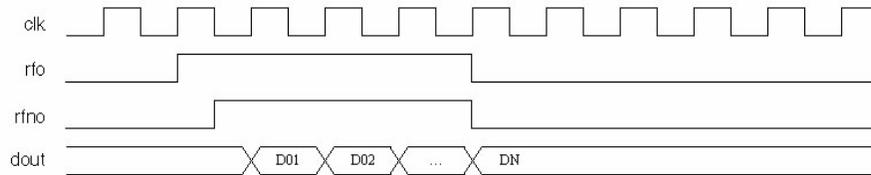
Note: Signals are transferred on the rising edge. N is the block size.
