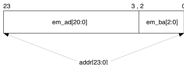
Figure 5. Mapping of User Address to Memory Address for Single Chip Select
